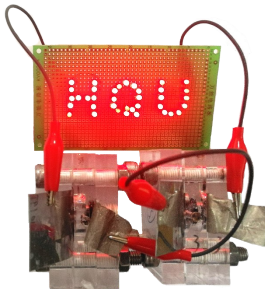
Fig. S16 Photograph of a light board consisting of 37 LEDs illuminated by two Zn-air batteries in series.
