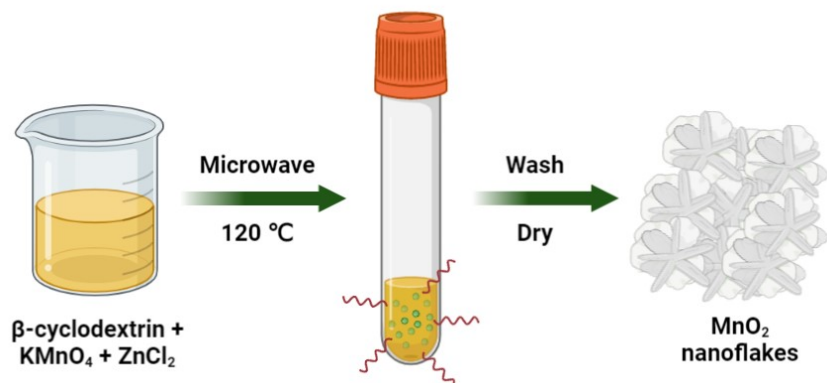
Figure S1. The simplified schematic fabrication process of Zn-doped \delta -MnO 2 .
