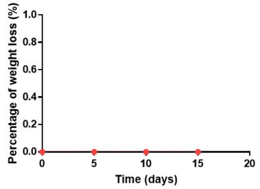
**Supplementary figure 8:** (a) Swelling ratio of PEO/PCL/JFA scaffold over a period of 240 hours (n=4) (b) Degradation profile by percentage of weight loss analysis of PEO/PCL/JFA scaffold over a period of 15 days (n=4)
