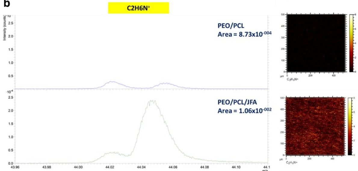
**Supplementary figure 6:** TOF-SIMS detection of  $\text{NH}_4^+$  (a) and  $\text{C}_2\text{H}_6\text{N}^+$  (b) for PEO/PCL, aminolyzed PEO/PCL, PEO/PCL/JFA and PEO/PCL/JFA scaffolds post incubation in water (37°C for 7 days). Peak area normalized to the ion intensity as well as ion map are shown for each condition.
