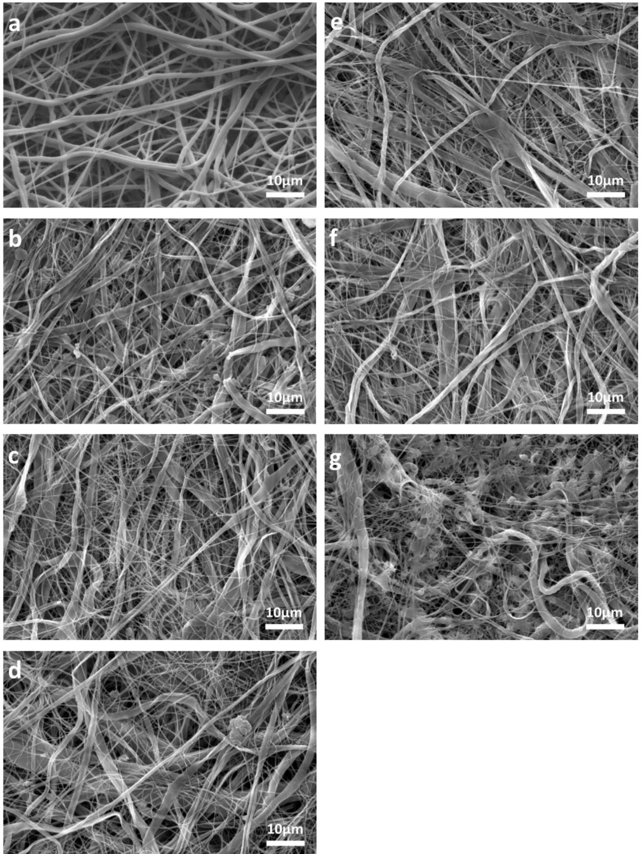
**Supplementary figure 3:** SEM image of PEO/ PCL scaffolds before (a) and after aminolysis treatments of 30min (b), 1h (c), 1h30 (d), 2h (e), 2h30 (f), 3h (g).
