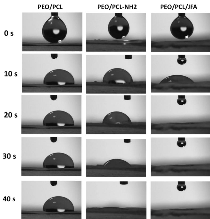
Supplementary figure 5: Images of water contact angle (WCA) measurement for PEO/PCL, aminolyzed PEO/PCL and PEO/PCL/JFA scaffolds.
