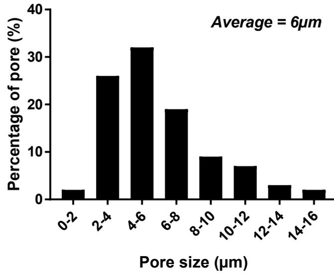
**Supplementary figure 2:** Histogram of PEO/PCL/JFA scaffold pore size distribution obtained from SEM images after cryosection of the scaffolds. The histograms were calculated from 100 measurements on Image J 1.52h software (from the ImageJ package Fiji) based upon five different SEM images.
