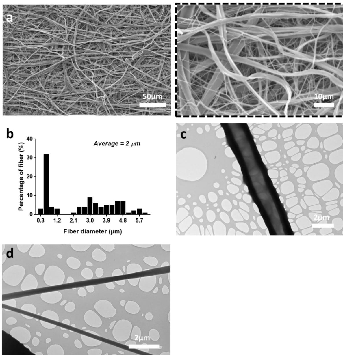
**Supplementary figure 1:** Morphology characterisation of PEO/PCL scaffold with PEO 400kDa including low and high magnification SEM images (a), the histogram of the fibre diameter distribution calculated from 100 measurements based upon five different SEM images (b) and of individual fibre morphology and structure using TEM (c). TEM image of PEO/PCL scaffold with PEO 900kDa is shown in (d) illustrating loss of the core/shell structure.
