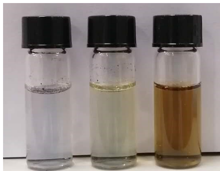
Fig. S3 The image of the sample solution from left to right is the aqueous solution of hemin, mixture of hemin and GOX, and GHN, indicating after hemin was polymerized onto GOX, it became soluble in aqueous solution.
