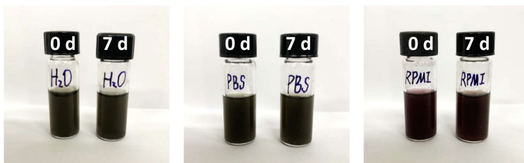
Fig. S8 The photographs of CFAP dispersed in H 2 O, PBS, and RPMI, respectively.
