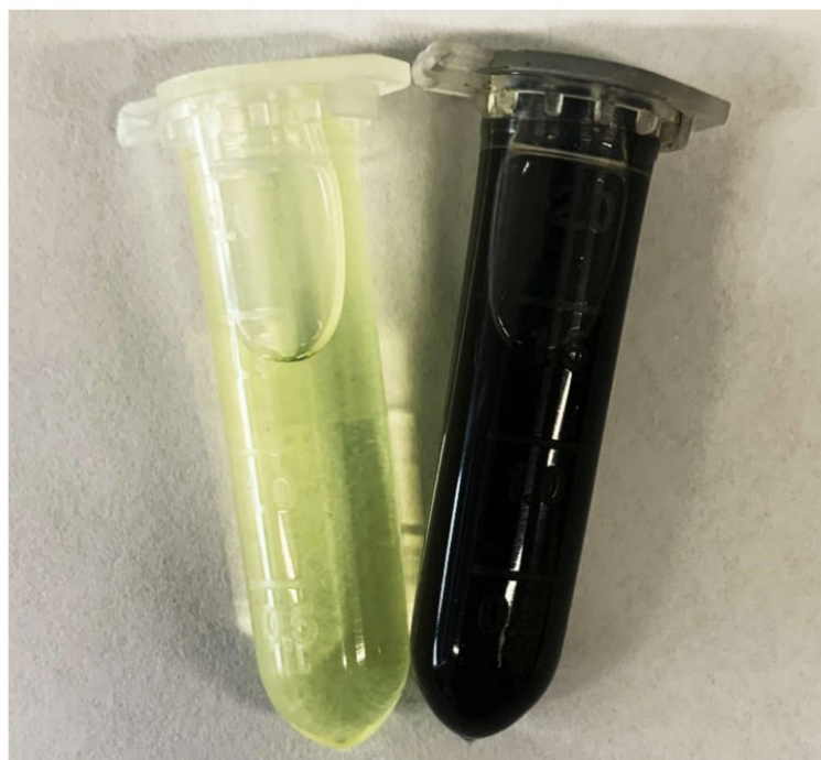
Fig. S9 Photographs of baicalein (left) and the as-synthesized Fe-BaP (right) in ethanol.
