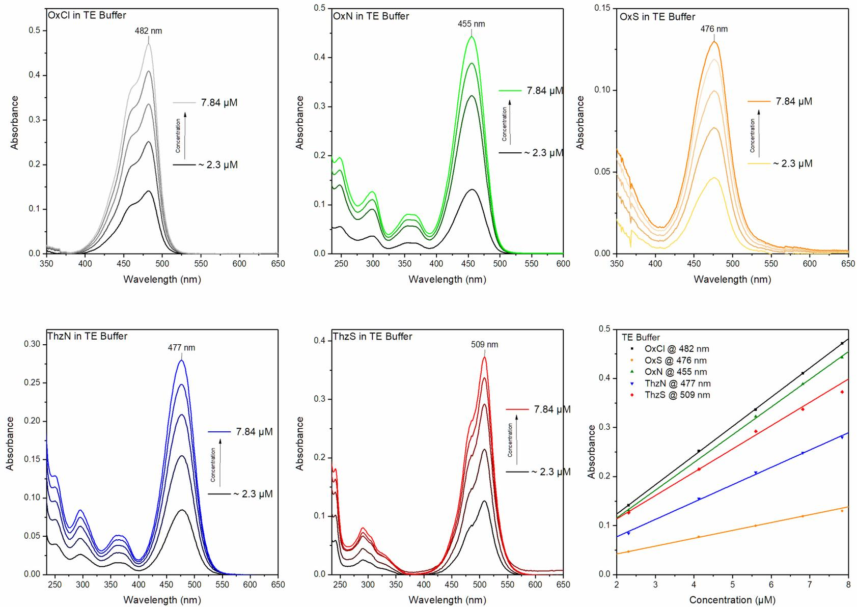
**Fig. S14.** UV-vis spectra of the synthesized dyes in five different concentrations in TE Buffer and linear fittings of the lowest energy maxima values.
