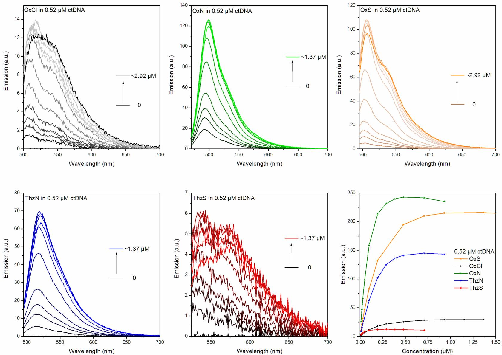
**Fig. S22.** Fluorescence spectra of the synthesized dyes with increasing concentration in 0.52  $\mu\text{M}$  ctDNA solution and the corresponding emission maxima plotted as the function of concentration.
