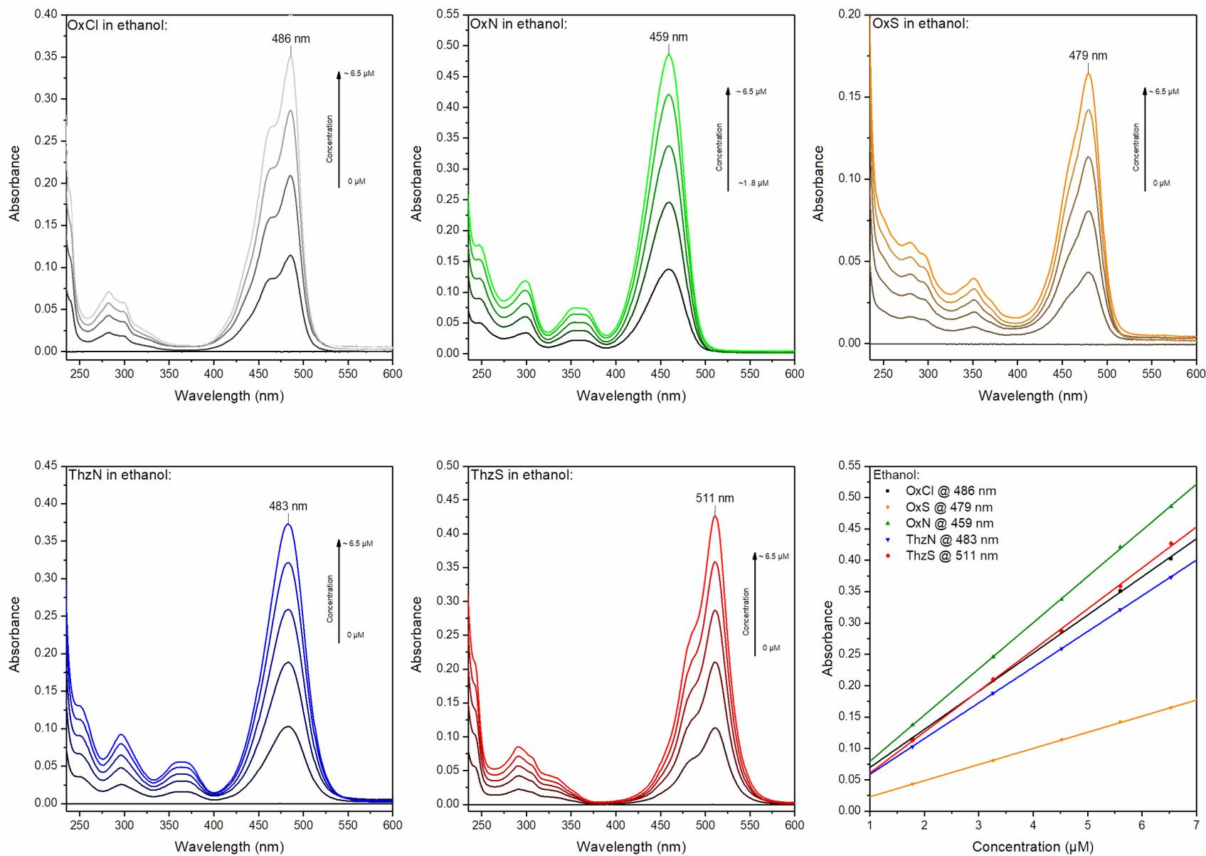
**Fig. S15.** UV-vis spectra of the synthesized dyes in five different concentrations in ethanol and linear fittings of the lowest energy maxima values.
