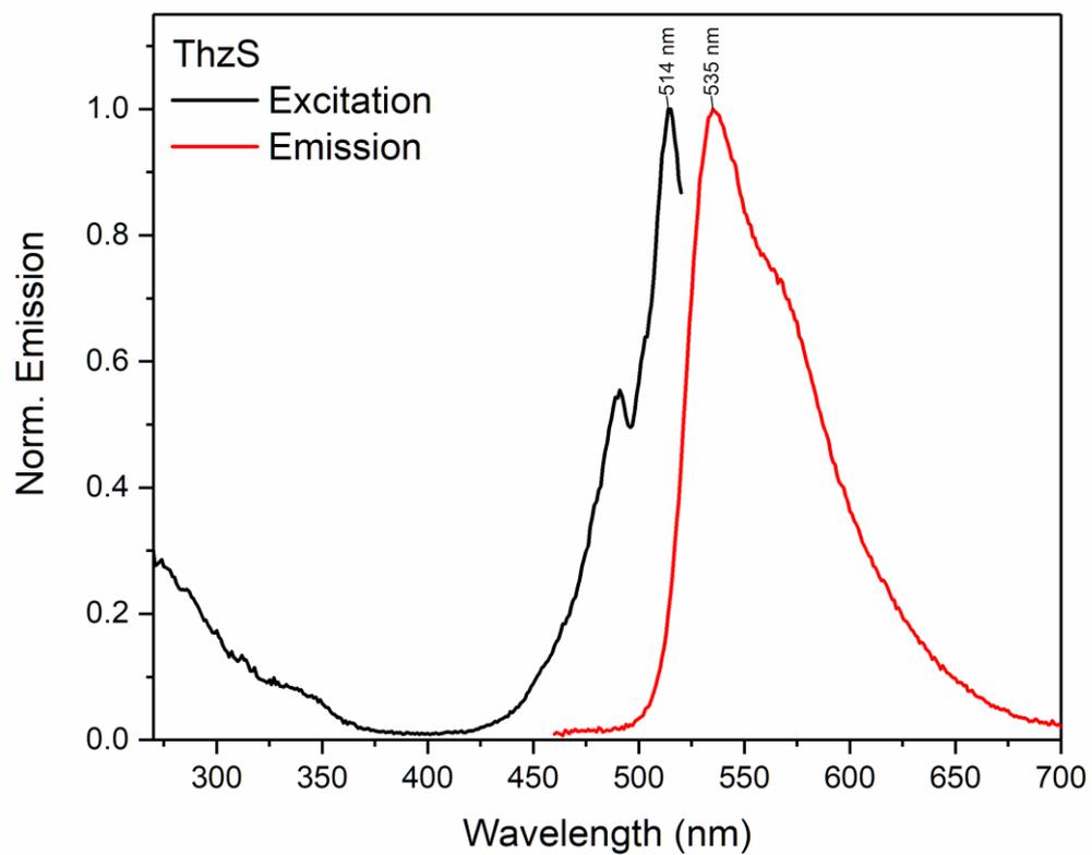
**Fig. S13.** Excitation and emission spectra of the ThzS **5** dye in binding with ctDNA in TE buffer.
