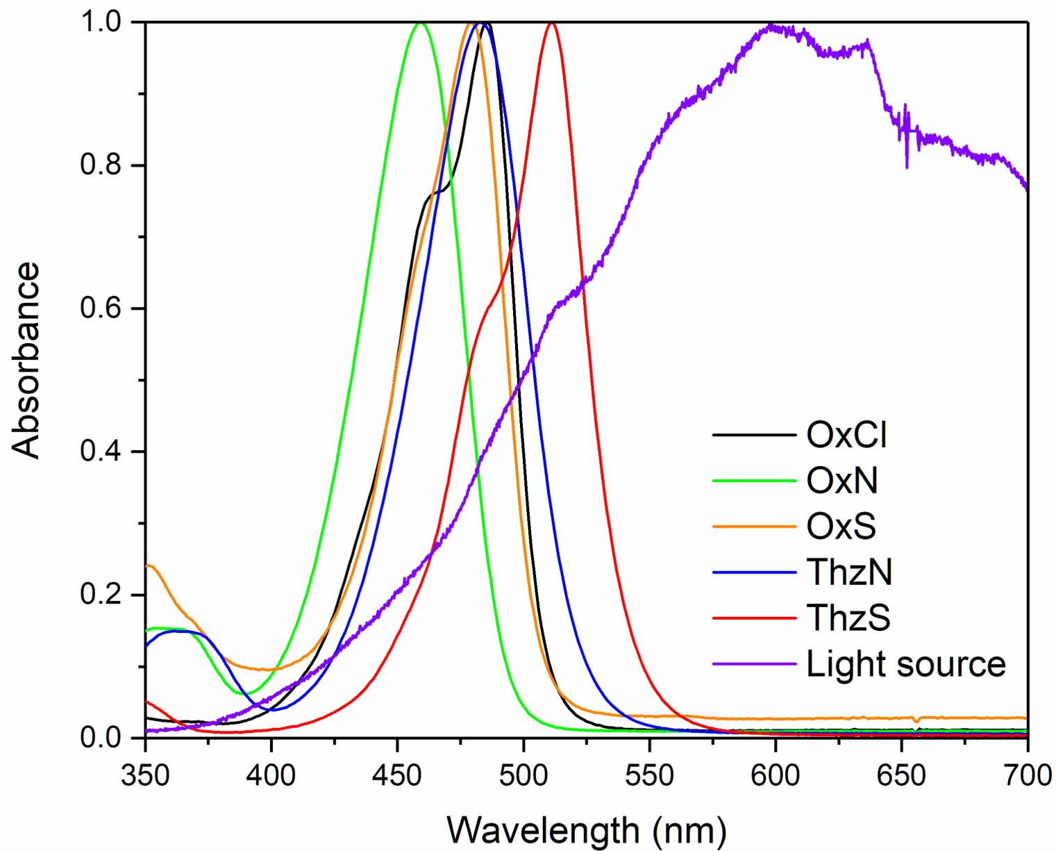
**Fig. S19.** Absorption spectra of the synthesized dyes overlaid with the 3300 K halogen lamp light source used for the photobleaching experiments.
