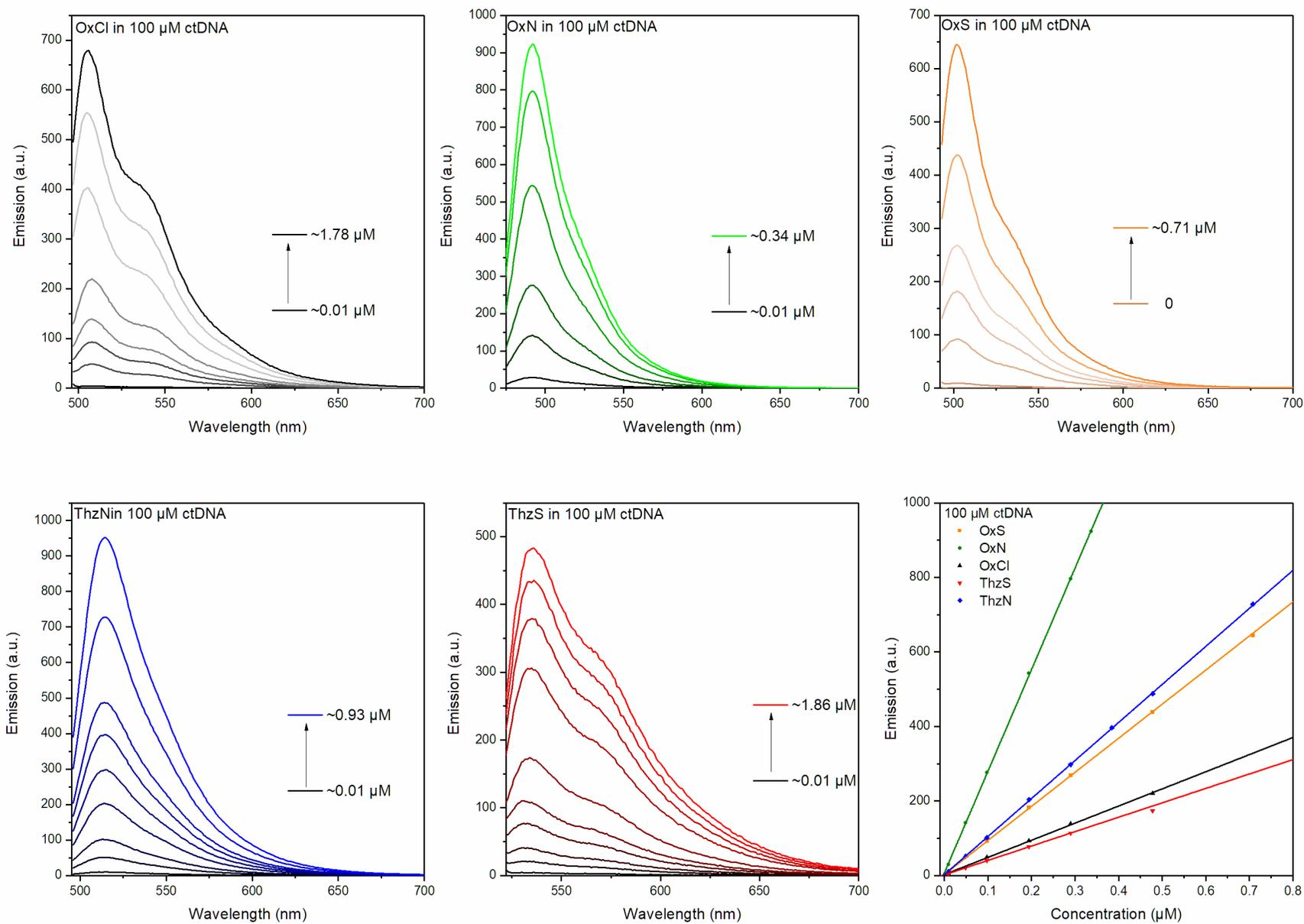
**Fig. S23.** Fluorescence spectra of the synthesized dyes with increasing concentration in 100  $\mu\text{M}$  ctDNA solution and the corresponding emission maxima plotted as the function of concentration.
