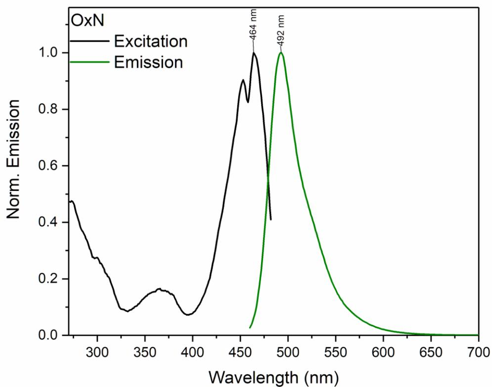
**Fig. S10.** Excitation and emission spectra of the OxN 2 dye in binding with ctDNA in TE buffer.
