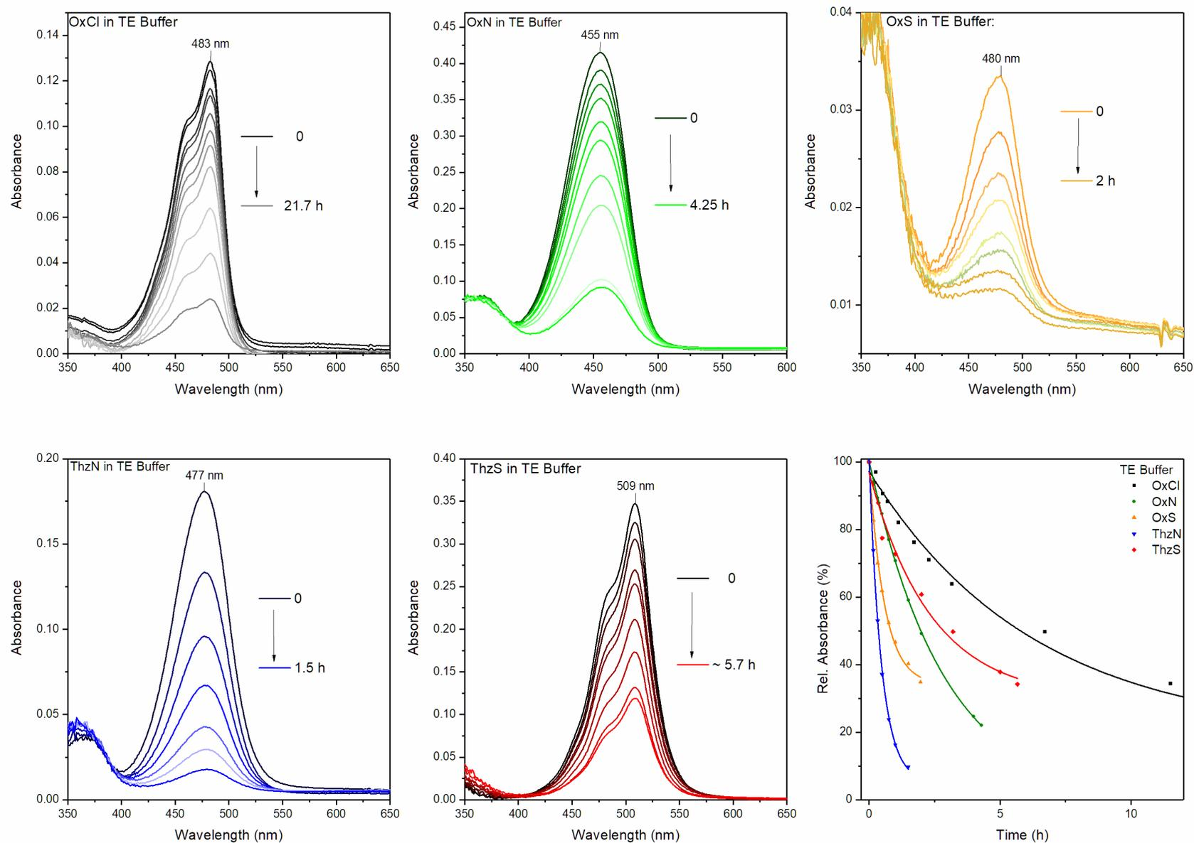
**Fig. S20.** Recorded absorption spectra of the synthesized dyes under a  $22 \text{ mW/cm}^2$  halogen lamp exposure over time in TE buffer. Fitting exponential decay function to the lowest energy maxima values gave  $t_{1/2}$  values for each dye.
