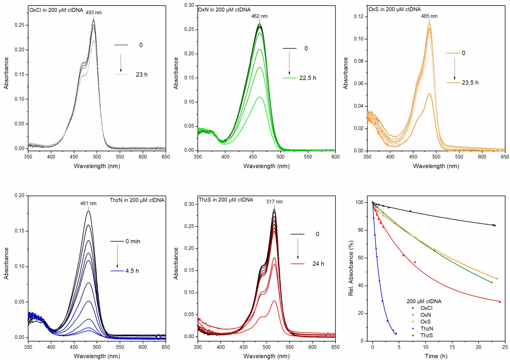
**Fig. S21.** Recorded absorption spectra of the synthesized dyes under a 22 mW/cm<sup>2</sup> halogen lamp exposure over time in 200 μM ctDNA. Fitting exponential decay function to the lowest energy maxima values gave  $t_{1/2}$  values for each dye.
