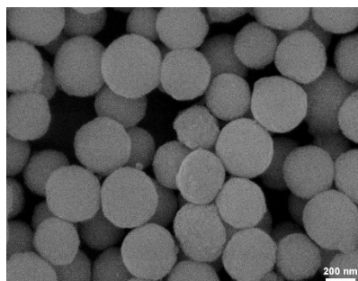
Fig. S4 SEM image of the \text{Cu}_3(\text{PO}_4)_2 after five cycles of on-off laser irradiation procedure (808 nm, 2.0 W/cm 2 ).
