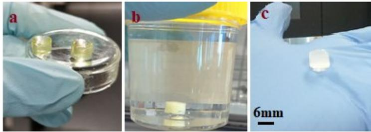
Figure S6. Cylinder samples for compression tests: (a) after photocrosslinking, (b) immersing in PBS, (c) swollen samples for compression test.
