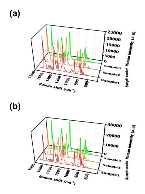
under repeated temperature changes from 25 °C to 50 °C for 3 cycles. Figure S1. SERS spectra of three different batches of MGITC-encoded GNRCs in (a) SBS and
