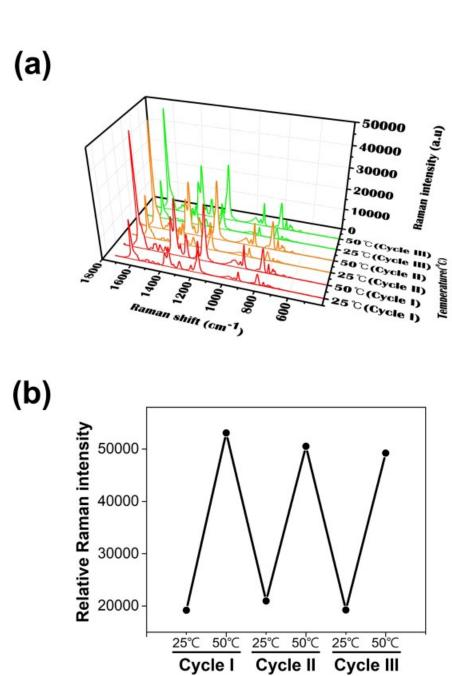
Figure S2. Relative Raman spectra and Raman intensity of JRCPCs with GNRCs in ETE configuration under repeated temperature changes from 25 °C to 50 °C for 3 cycles.
