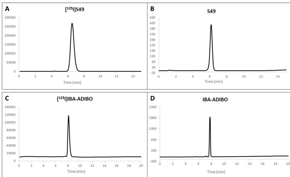
**Figure S2.** Analytical radio-HPLC chromatograms of purified [<sup>125</sup>I]S49 (A) and [<sup>125</sup>I]IBA-ADIBO (C) compared to analytical UV-HPLC chromatograms of non radioactive references S49 (B) and IBA-ADIBO (D). Radio-HPLC detector was connected in series after the UV detector accounting for the slight difference of retention times ( $\approx$  0.3 min) observed between <sup>125</sup>I and <sup>127</sup>I products.
