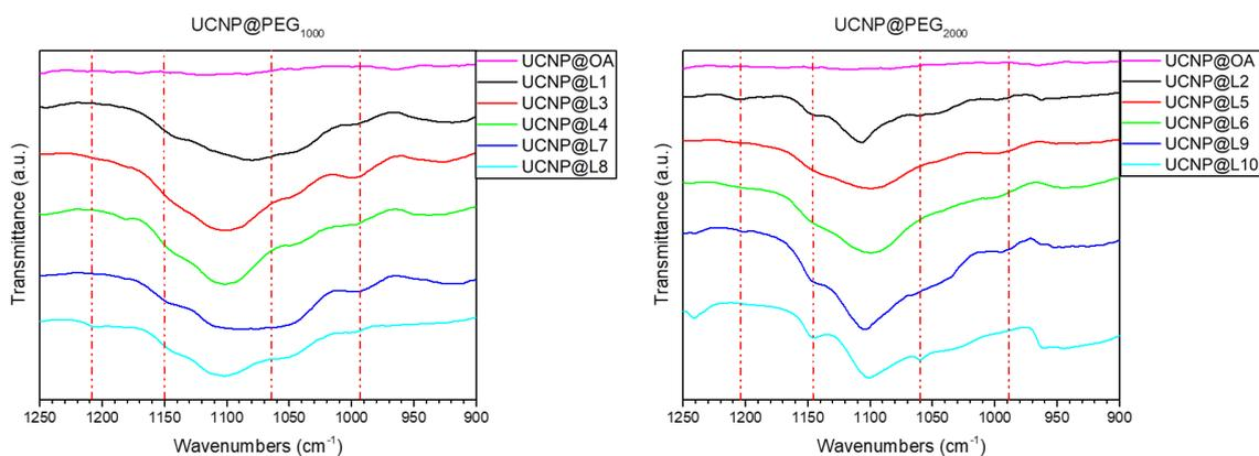
**Figure S5:** ATR-FTIR spectra of UCNP@OA and UCNP@L(1-10), zoom in the range of 900-1250 cm<sup>-1</sup>. Red dashed lines highlight P=O and P-O bands not or faintly visible in the spectra.
