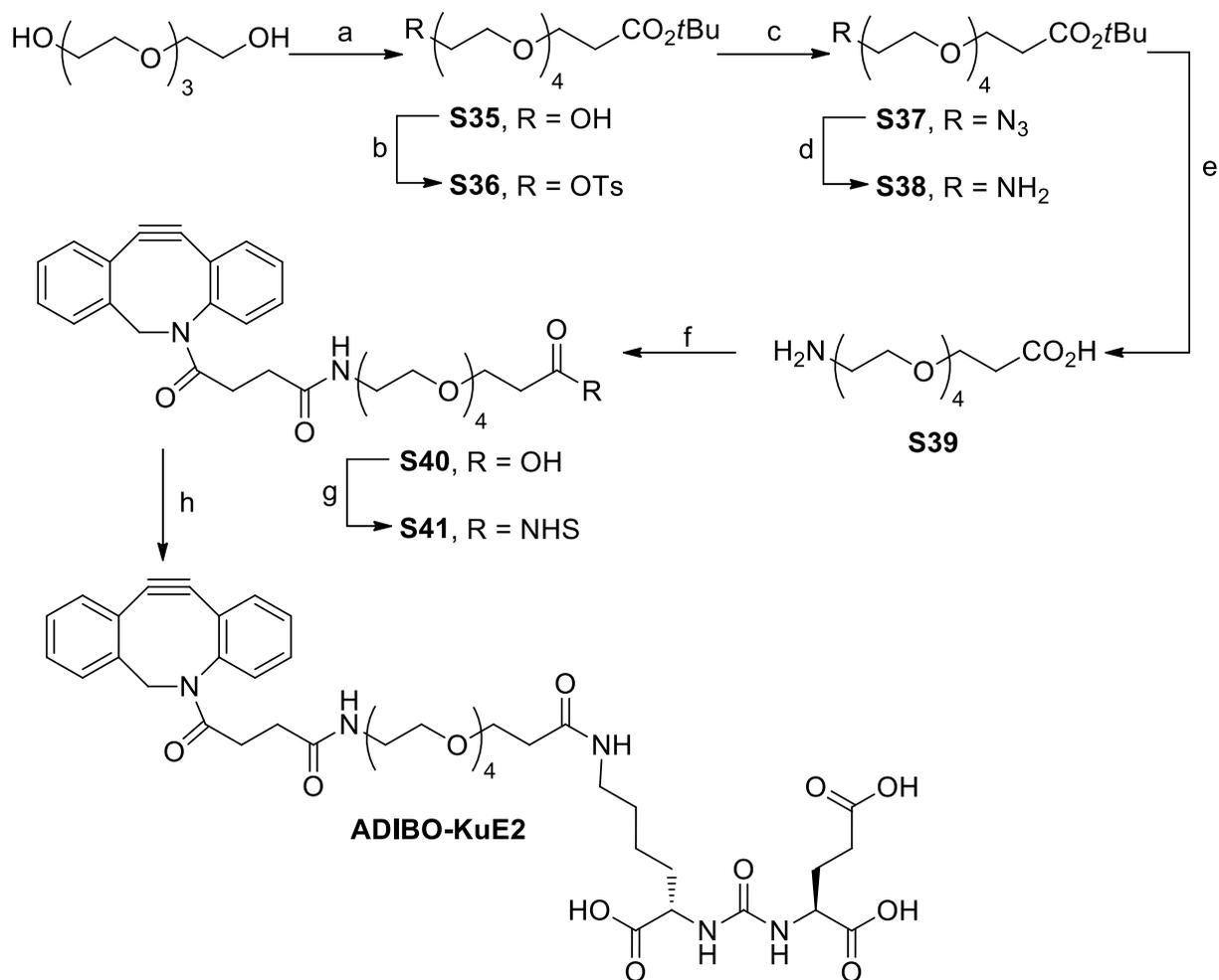
**Reaction conditions:** a) NaH (60 wt% in mineral oil), *tert*-butyl acrylate, THF, RT; b) TsCl, pyridine, RT; c)  $NaN_3$ , DMF, RT then 55 °C; d)  $PPh_3$ ,  $Et_2O$ ,  $H_2O$ , RT; e) TFA, anisole,  $CH_2Cl_2$ , 0 °C then RT; f) S34, DIPEA, DMF, RT; g) NHS, EDC.HCl,  $CH_2Cl_2$ , RT; h) S32, DIPEA, DMF, RT
