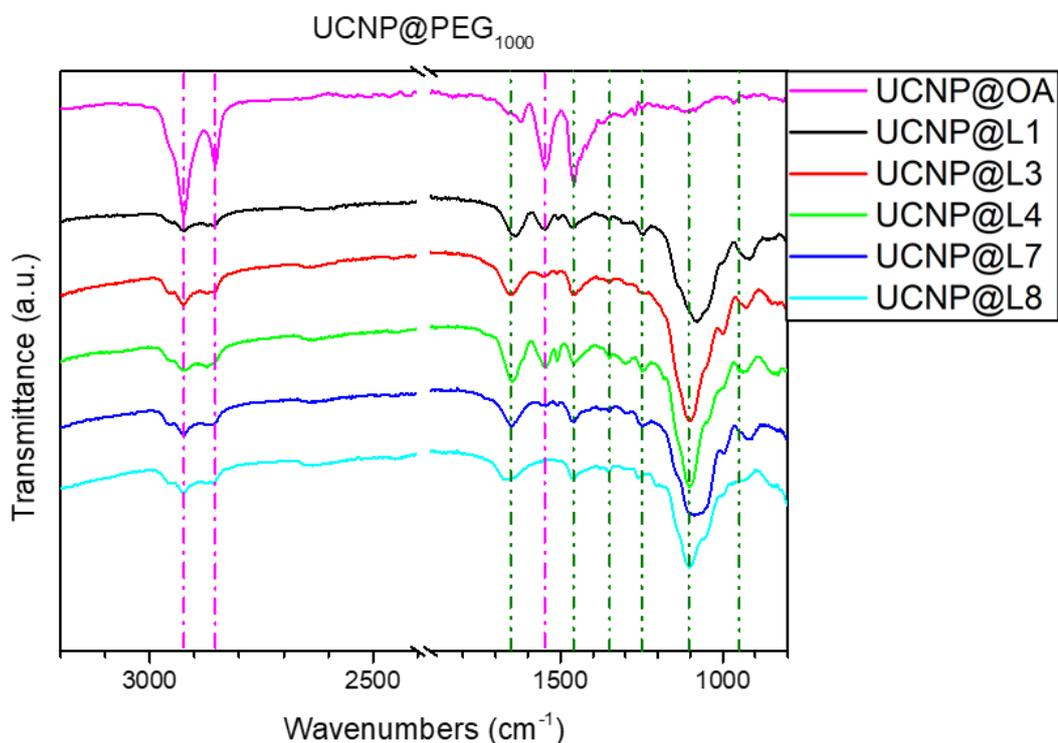
**Figure S4:** ATR-FTIR spectra of UCNP@OA and UCNP after ligand exchange with PEG<sub>(1000)</sub> ligands (UCNP@L1, L3, L4, L7 and L8). Magenta dashed lines highlight OA =C-H and C=O bands while green dashed lines highlight PEG backbone bands.
