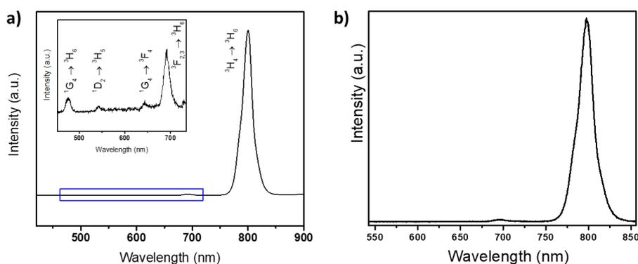
**Figure S7.** (a) Full UCL spectrum recorded upon 980 nm excitation from one-pot synthesized UCNPs, upper insert shows all the Tm<sup>3+</sup> transitions in the 450-750 nm range exhibiting a weak intensity in comparison with that of the  $^3H_4 \rightarrow ^3H_6$  transition at 800 nm; (b) UCL spectrum recorded from UCNP@L9 in deionized water upon excitation at 980 nm.
