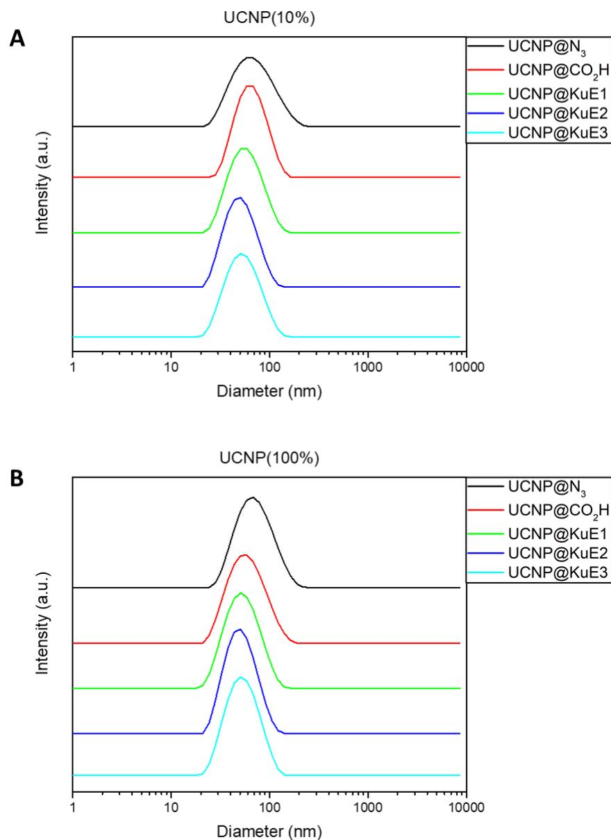
**Figure S10.** DLS analysis of particle-size distribution of UCNP@N<sub>3</sub>(10%) (A) and UCNP@N<sub>3</sub>(100%) (B) before and after SPAAC reaction with ADIBO-KuE(1-3) and ADIBO-CO<sub>2</sub>H S33 derivatives. Particle size was analysed using a diluted suspension of UCNP (1 mg/mL) in deionized water.
