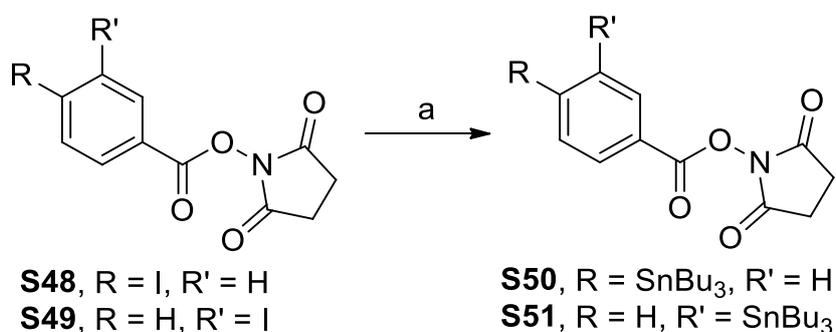
**Reaction conditions:** a) Sn<sub>2</sub>Bu<sub>6</sub>, Pd(PPh<sub>3</sub>)<sub>4</sub>, toluene, reflux.
