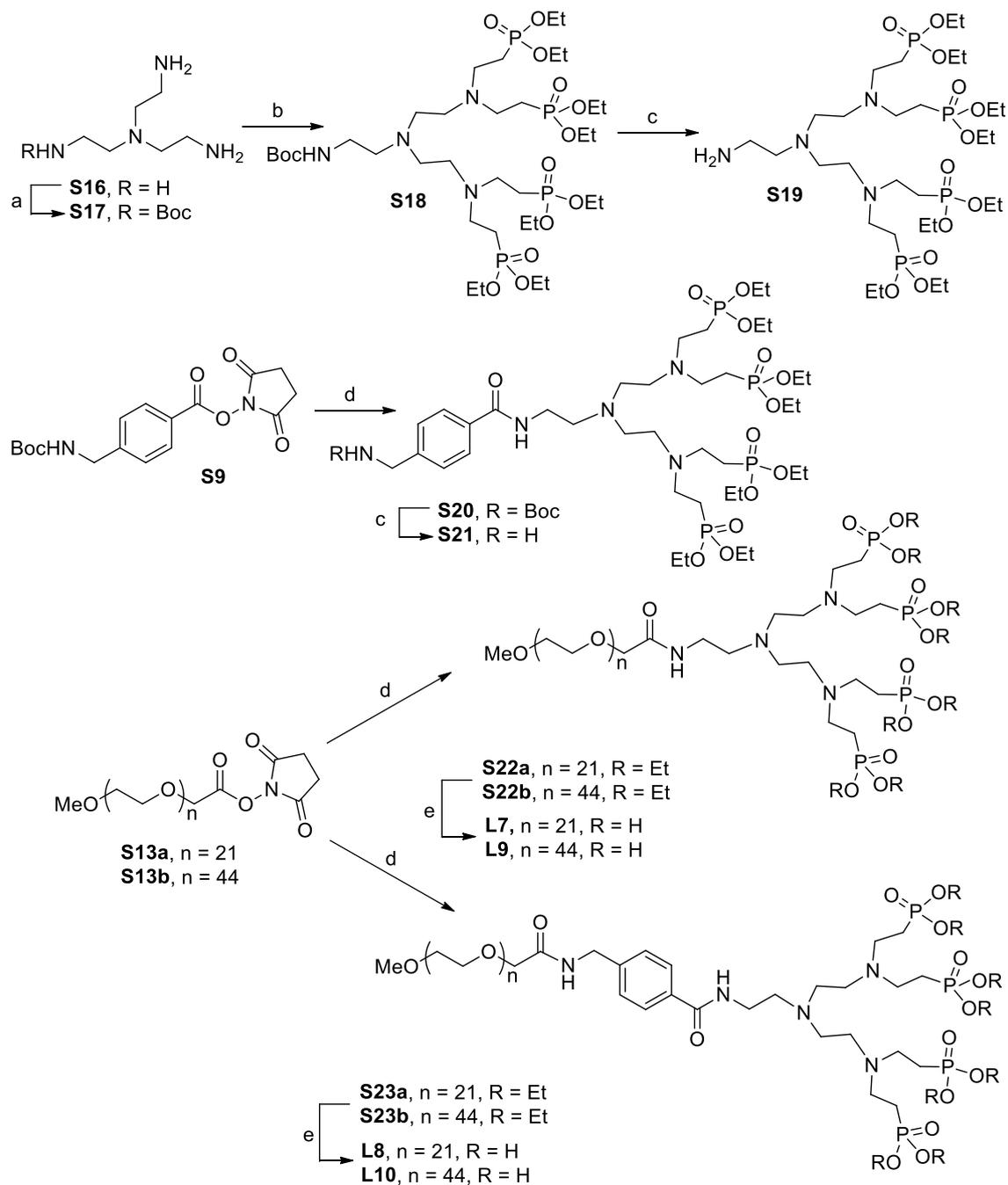
**Reaction conditions:** a)  $\text{Boc}_2\text{O}$ ,  $\text{CHCl}_3$ ,  $0^\circ\text{C}$  then RT; b) diethyl vinylphosphonate,  $\text{H}_2\text{O}$ , RT; c) TFA,  $\text{CH}_2\text{Cl}_2$ ,  $0^\circ\text{C}$ ; d) appropriate amine (**S19** or **S21**), DIPEA, DMF, RT; e) (i) TMSBr,  $0^\circ\text{C}$  then RT; (ii) MeOH, RT.
