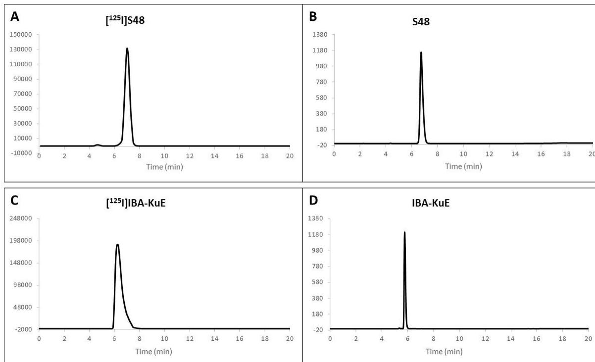
**Figure S1.** Analytical radio-HPLC chromatograms of purified [<sup>125</sup>I]S48 (A) and [<sup>125</sup>I]IBA-KuE (C) compared to analytical UV-HPLC chromatograms of non radioactive references S48 (B) and IBA-KuE (D). Radio-HPLC detector was connected in series after the UV detector accounting for the slight difference of retention times ( $\approx 0.3$  min) observed between <sup>125</sup>I and <sup>127</sup>I products.
