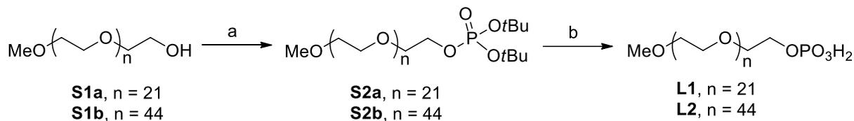
**Reaction conditions:** a) (i)  $(i\text{Pr})_2\text{NP}(\text{OtBu})_2$ , tetrazole,  $\text{CH}_2\text{Cl}_2$ , RT; (ii) mCPBA, RT; b) HCl 2N,  $\text{Et}_2\text{O}$ , 0 °C then RT.
