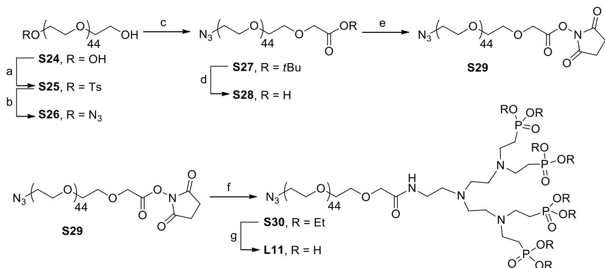
**Reaction conditions:** a) TsCl, TEA,  $\text{CH}_2\text{Cl}_2$ , 0 °C; b)  $\text{NaN}_3$ , DMF, 90 °C; c) (i) NaH, THF, 0 °C; (ii)  $\text{BrCH}_2\text{CO}_2t\text{Bu}$ , 50 °C; d) aq. HCl 2N, reflux; e) NHS, DCC,  $\text{CH}_2\text{Cl}_2$ , 0 °C then RT; f) **S19**, DIPEA, DMF, RT; g) (i) TMSBr, 0 °C then RT; (ii) MeOH, RT.
