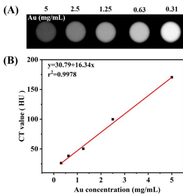
**Fig. S9** In vitro CT images (A) and CT value (HU) (B) of PMC@AuNP as a function of the Au concentration.
