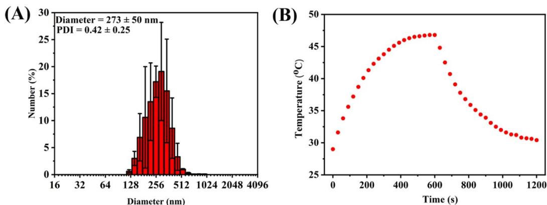
**Fig. S4** (A) the DLS-determined diameter and (B) NIR-II-mediated heating-cooling curve of the bigger aggregates formed from the unimers of amphiphilic copolymers with  $\text{HAuCl}_4$ .
