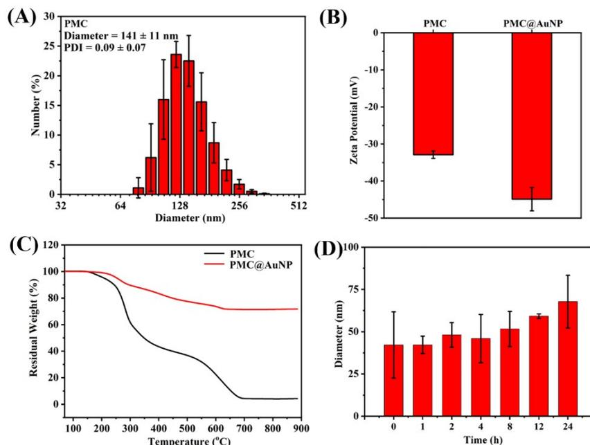
**Fig. S3** (A) The DLS-determined diameter of PMC micelle; (B) Zeta potentials and (C) TGA curves of PMC micelle and PMC@AuNP; (D) Hydrodynamic diameter of PMC@AuNP over incubation time when incubated in 10% FBS at 37 °C (n = 3).
