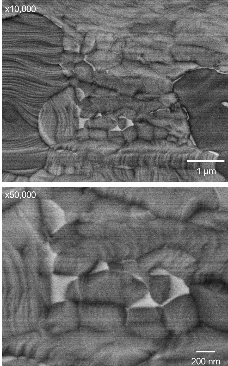
Figure S1. Backscattered electron (BSE) images of the non-treated Ti-6Al-4V film used in this study
