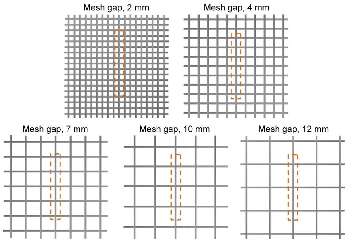
**Fig. S2** Schematic representation of the cutting strategies for typical rectangular piece specimens from corresponding RASF scaffolds. The dashed lines only represent the relative cutting positions compare to the underneath meshes (solid lines).
