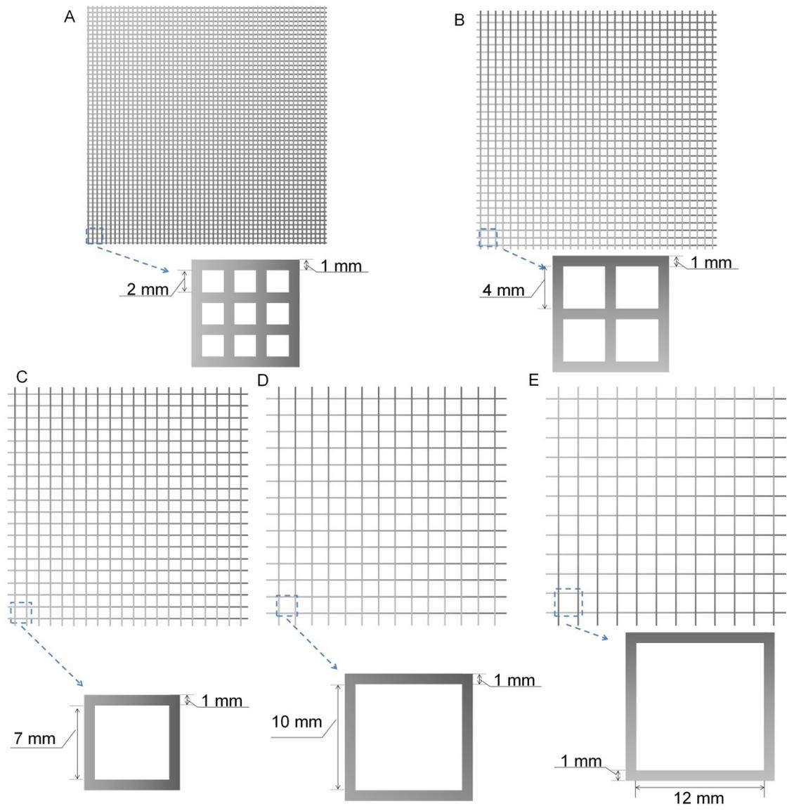
**Fig. S1** Schematic representation of mesh collectors with varied gap sizes. (A) 2 mm, (B) 4 mm, (C) 7 mm, (D) 10 mm and (E) 12 mm.
