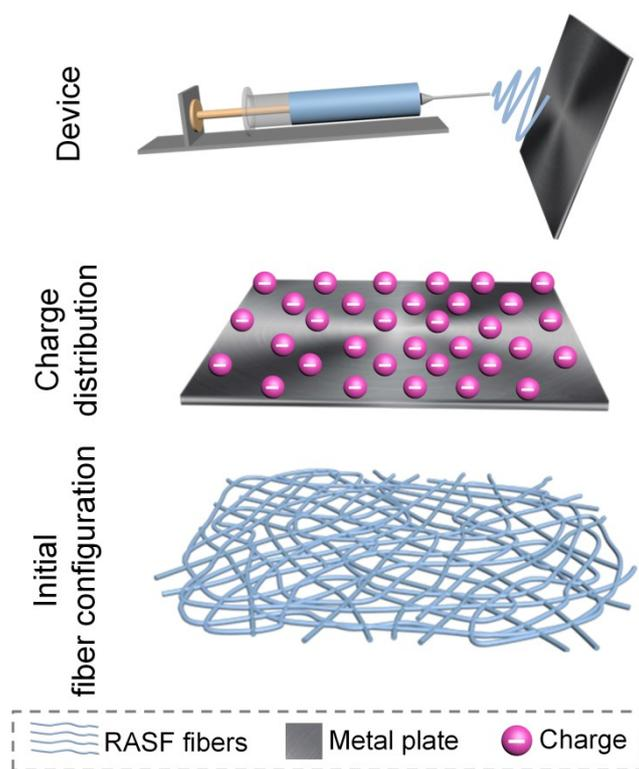
**Fig. S4** Schematic representation of the electrospinning device, charge distribution on traditional intact plate collector and corresponding configuration of initial electrospun RASF fibers.
