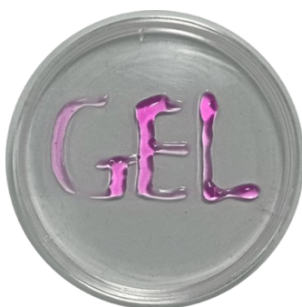
Fig. S2 Gel patterns formed by the injectable TP hydrogel containing rhodamine B
