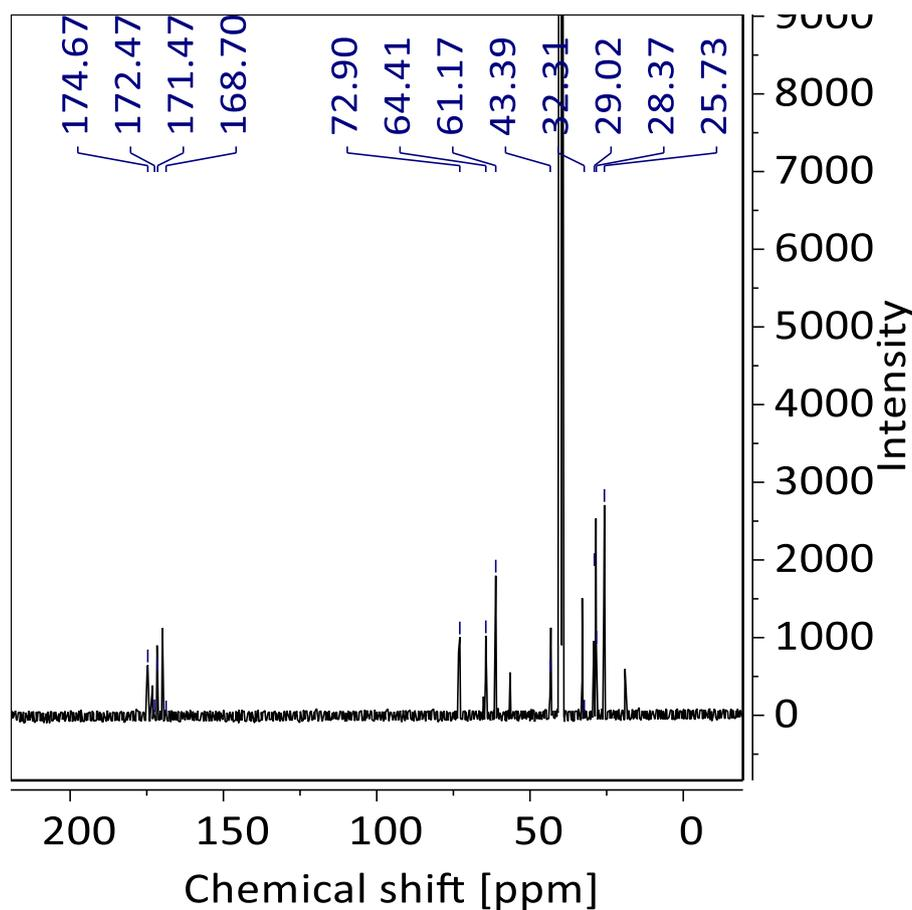
**Figure S10.** <sup>13</sup>C spectrum for POC\_1:1 prepolymer.
