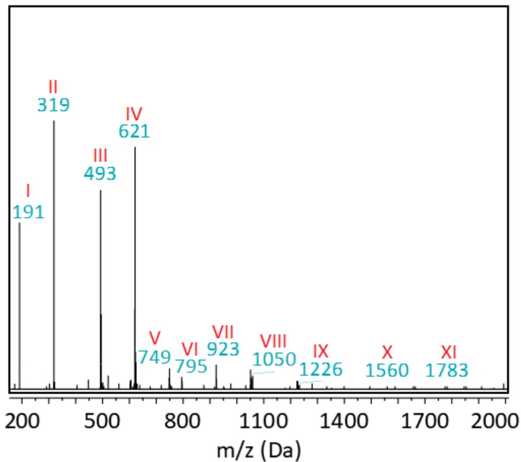
**Figure S7.** Mass spectrum of POC\_2:3 prepolymer obtained after 60 min of reaction, acquired via FIA-MS analysis (ESI). Ion labels are referred in the table below.
