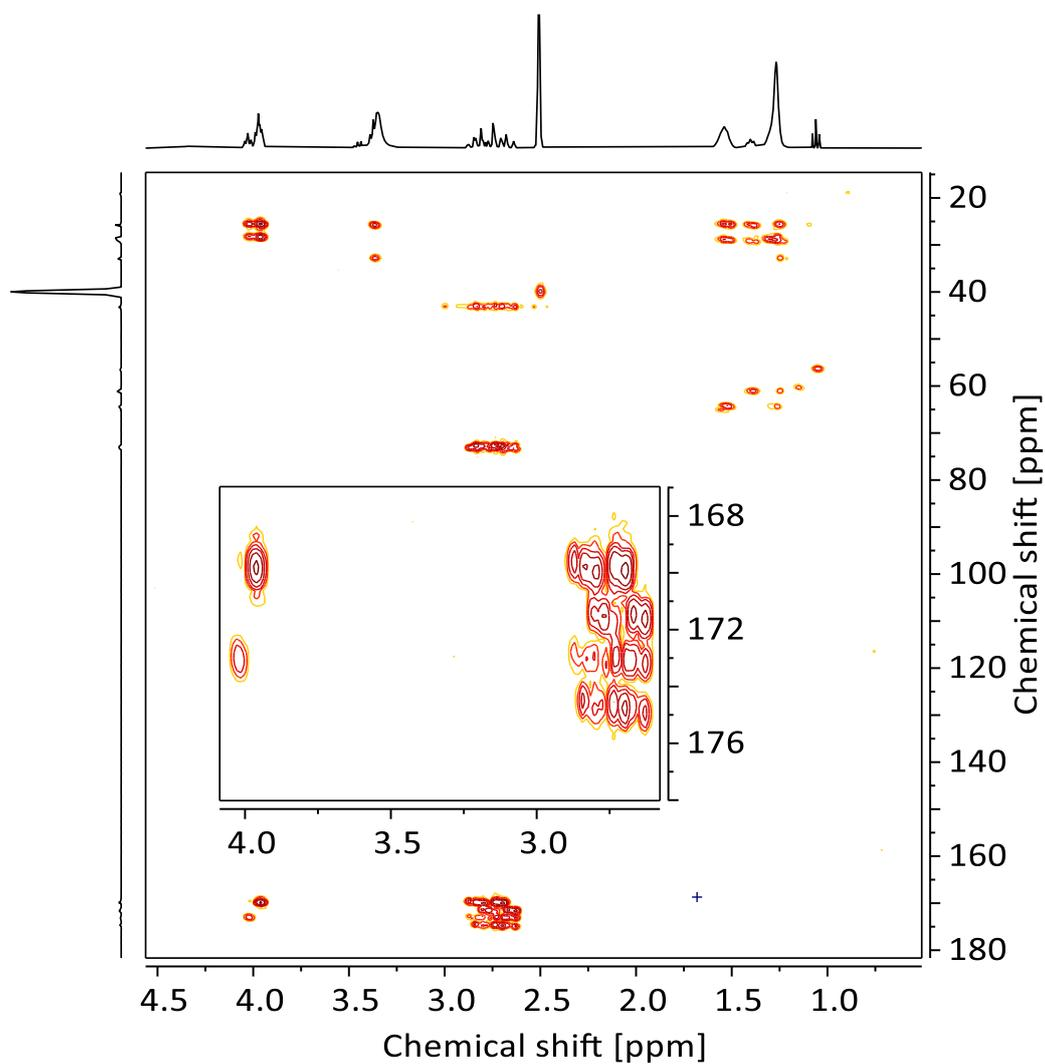
**Figure S13.**  $^1\text{H}$ - $^{13}\text{C}$  HMBC spectrum for POC\_1:1 prepolymer. Signals from correlations in carboxyl region were enlarged.
