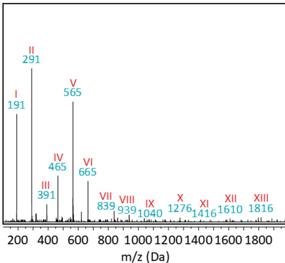
**Figure S6.** Mass spectrum of PHC<sub>2:3</sub> prepolymer obtained after 90 min of reaction, acquired via FIA-MS analysis (ESI). Ion labels are referred in the table below.
