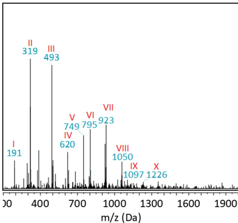
**Figure S2.** Mass spectrum of POC\_1:1 prepolymer acquired via FIA-MS analysis (ESI<sup>-</sup>). Ion labels are referred in the table below.
