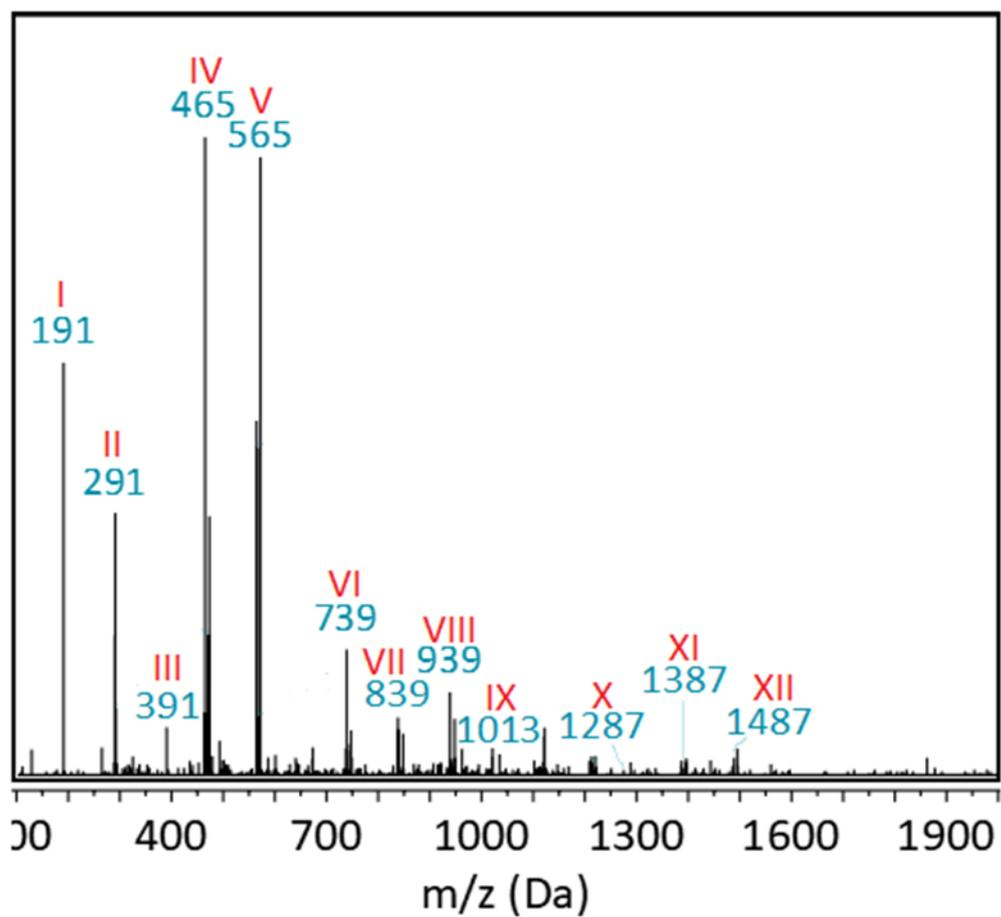
**Figure S3.** Mass spectrum of PHC<sub>1:1</sub> prepolymer acquired via FIA-MS analysis (ESI<sup>-</sup>). Ion labels are referred in the table below.
