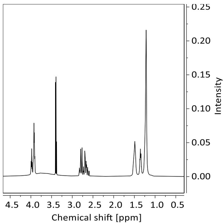
**Figure S16.** <sup>1</sup>H NMR Spectrum for POC<sub>2:3</sub> prepolymer obtained after 60 min of polycondensation.
