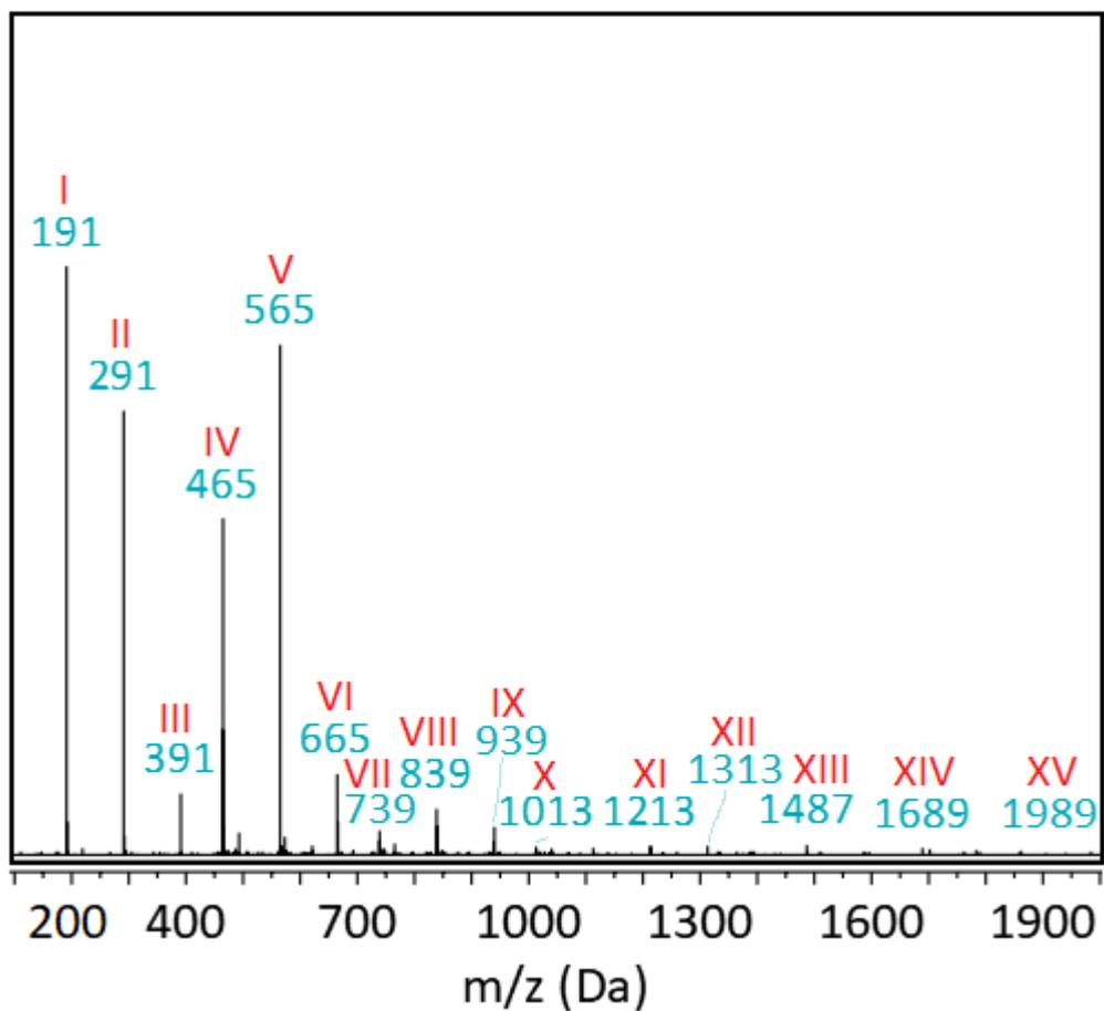
**Figure S5.** Mass spectrum of PHC<sub>2:3</sub> prepolymer obtained after 60 min of reaction, acquired via FIA-MS analysis (ESI). Ion labels are referred in the table below.
