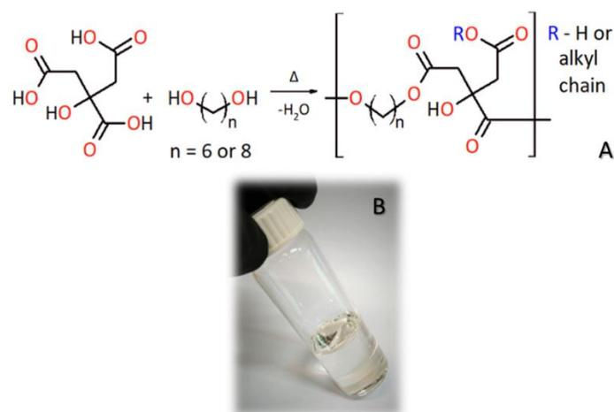
**Figure S1.** Synthesis scheme of PAC prepolymer fabrication (A) and the appearance of the final product (B).
