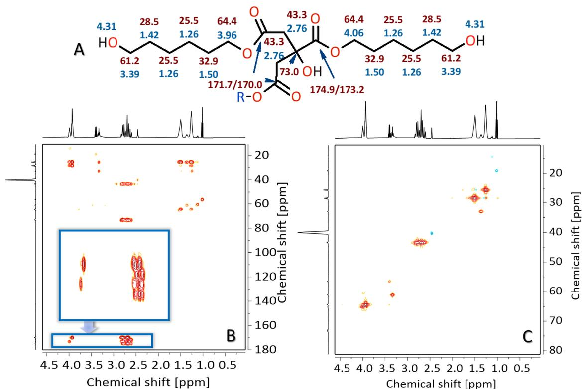
**Figure S14.** (A) Fragment of PHC prepolymer structure along with assignments of chemical shifts (crimson-carbons, blue-protons) based on NMR analysis. (B) HMBC spectra of PHC\_1:1 prepolymer with expanded proton-carbon correlation in carboxyl region. (C) HSQC spectra of PHC\_1:1 prepolymer.
