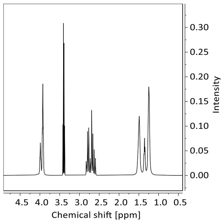
**Figure S18.** <sup>1</sup>H NMR Spectrum for PHC<sub>2:3</sub> prepolymer.
