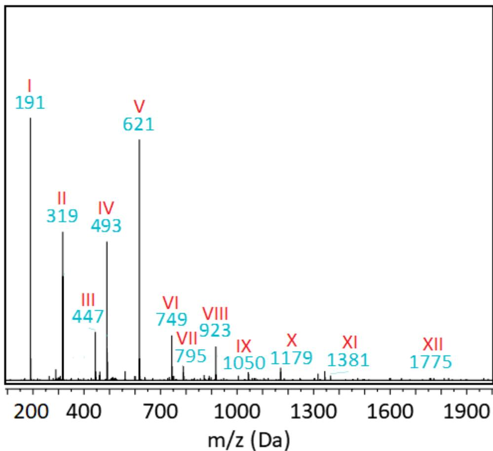
**Figure S8.** Mass spectrum of POC\_2:3 prepolymer obtained after 90 min of reaction, acquired via FIA-MS analysis (ESI). Ion labels are referred in the table below.
