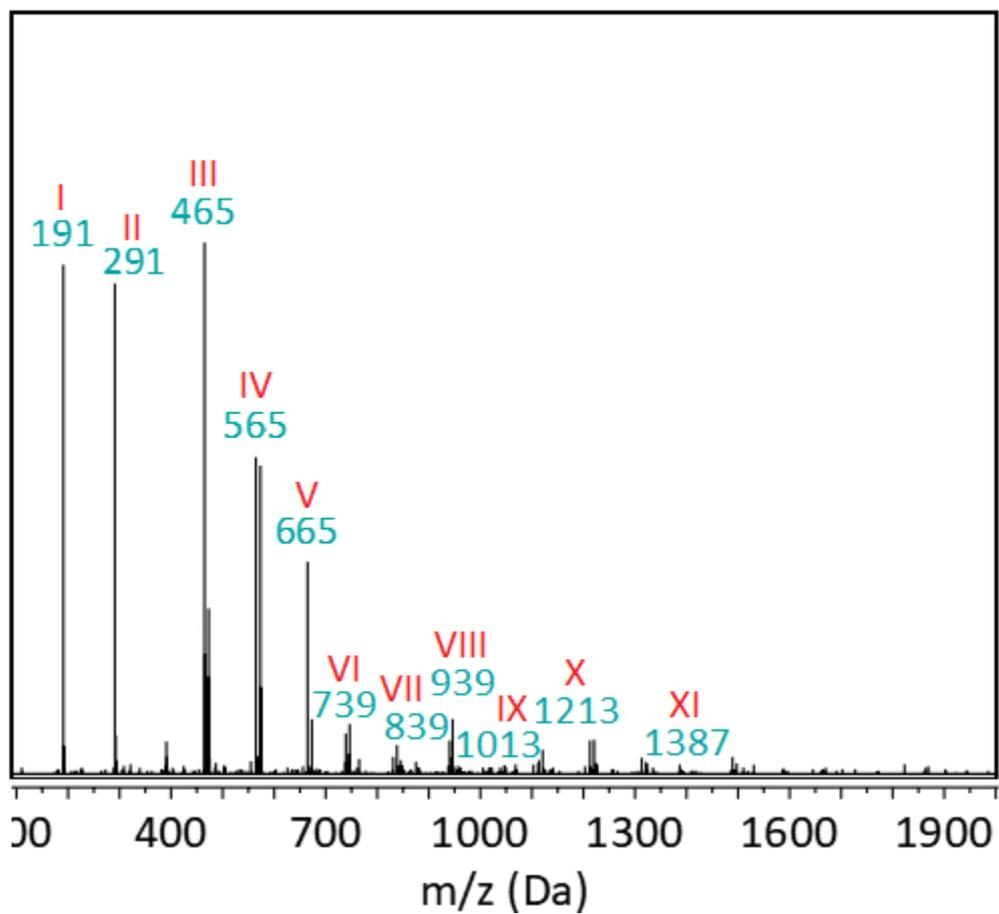
**Figure S4.** Mass spectrum of PHC<sub>2:3</sub> prepolymer acquired via FIA-MS analysis (ESI). Ion labels are referred in the table below.
