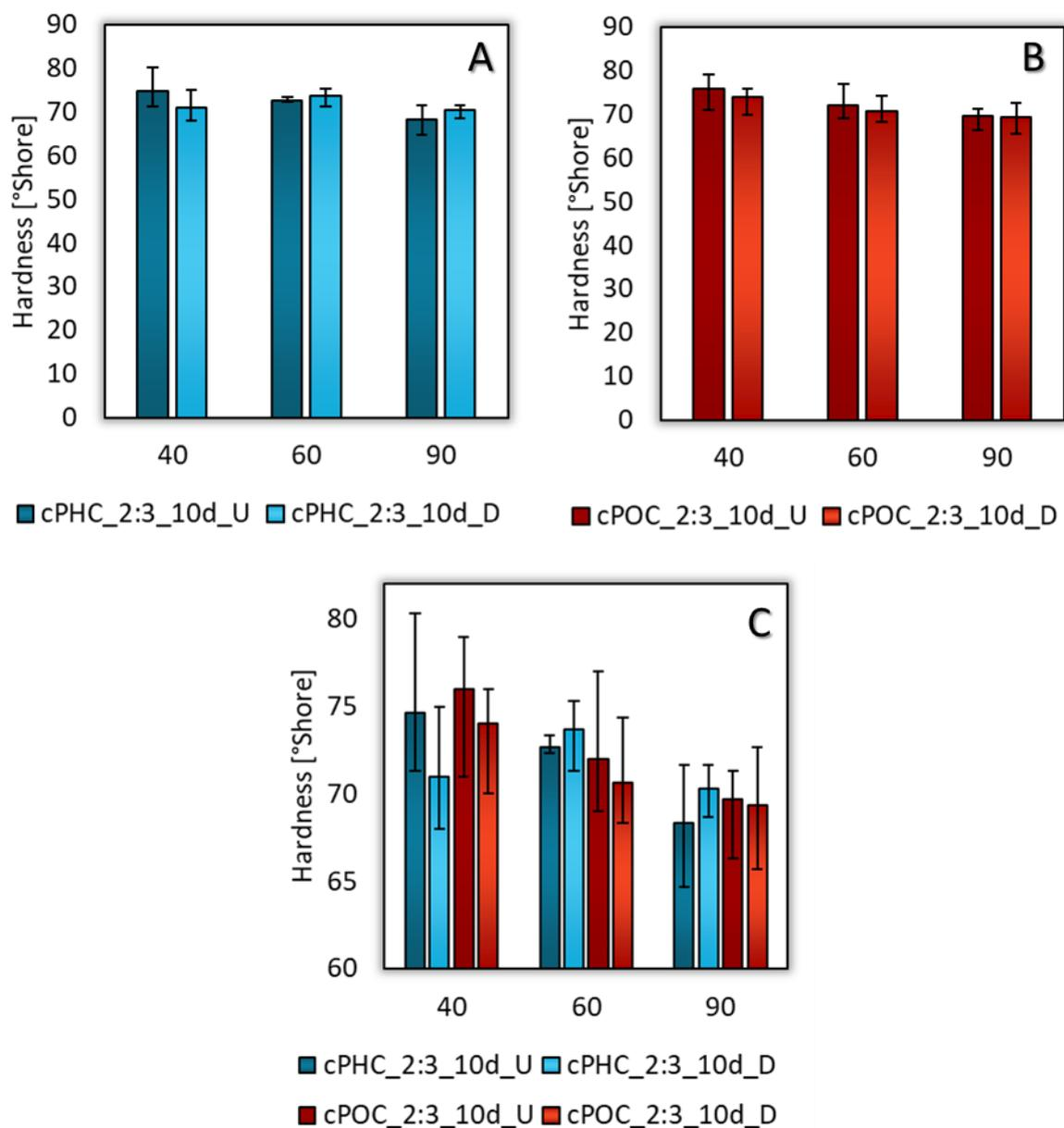
**Figure S22.** Graphs of hardness of cPAC\_2:3 materials obtained in various reaction times, **A** – cPHC materials, **B** – cPOC materials, and closeup of their comparison.
