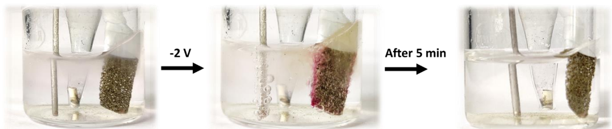
Figure S12A. Images displaying change of pH by applying -2\text{ V} in 0.1\text{ M} PBS (pH 7.4) solution containing 5\text{ }\mu\text{L} of 5% phenolphthalein (in ethanol) in the electrochemical cell; CE: Pt wire, RE: double junction Ag/AgCl/3 M KCl.
