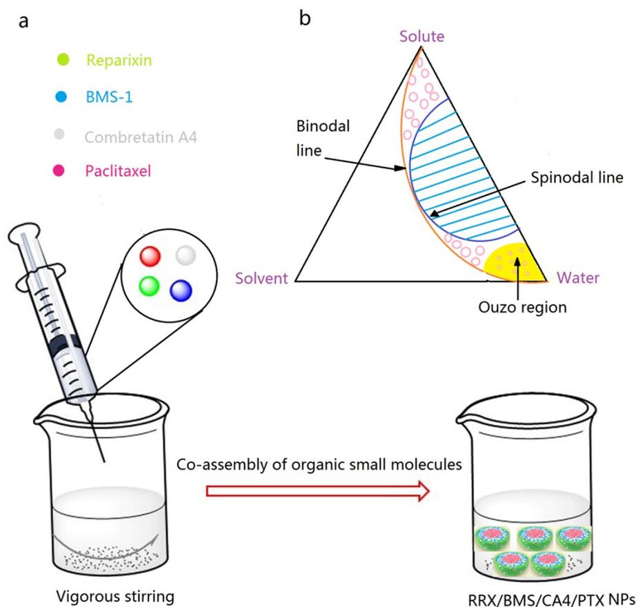
Fig. S1 Schematic illustration of preparation process of RRX/BMS/CA4/PTX NPs (a) and phase diagram of ternary solute/solvent/water (b).
