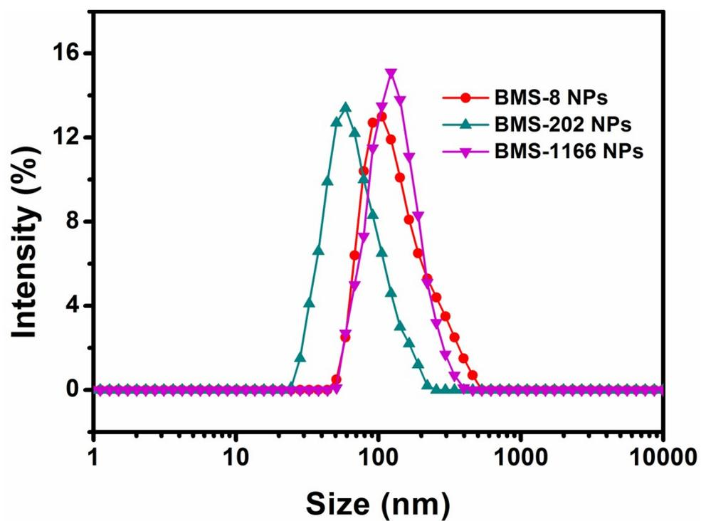
Fig. S5 DLS measurements of size of the BMS-8, BMS-202 and BMS-1166 NPs.
