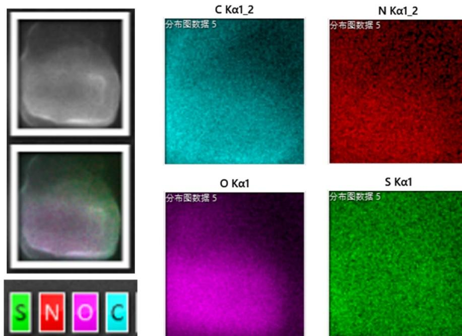
Fig. S2 SEM image and mapping images of RRX/BMS/CA4/PTX NP by SEM.
