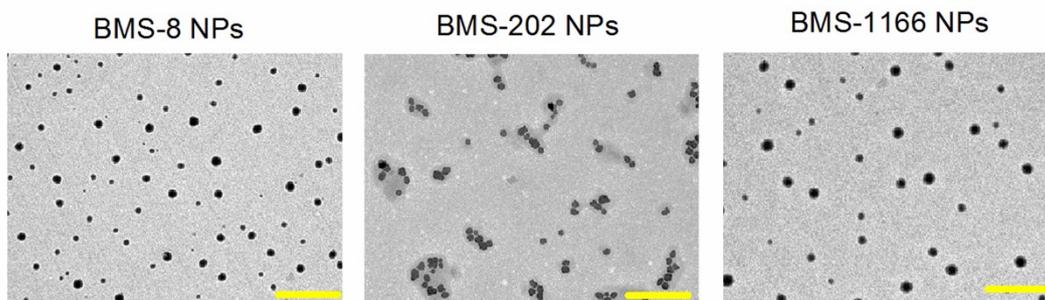
Fig. S4 TEM images of BMS-8, BMS-202 and BMS-1166 NPs ( scale bar = 500 nm).
