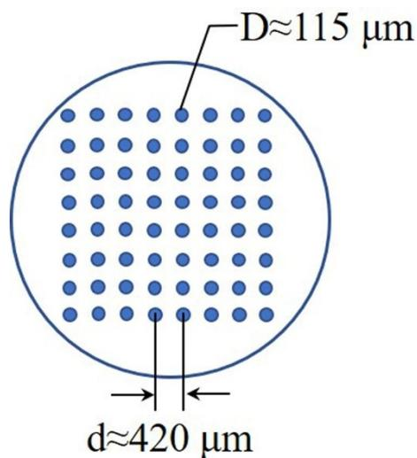
**Figure S1.** Pattern of laser texture on the YSZ coating surface.
