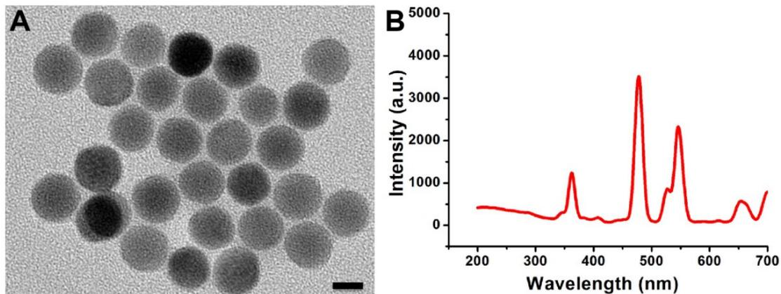
**Figure S1.** Characterization of the Tm/Er doped naked UCNPs ( $\text{NaYF}_4$ : Tm/Er,Yb). A) TEM imaging of the Tm/Er doped UCNPs. The size of UCNPs was about 30 nm. Scale bar: 20 nm. B) Fluorescent emission spectrum of the Tm/Er doped UCNPs. The UCNPs showed a strong fluorescent emission with 365/475/545/647 nm under the 980 nm NIR irradiation ( $1 \text{ W/cm}^2$ ).
