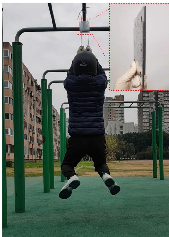
Figure S10. The bonded metal sheets with the bonding area of 10 \times 8 \text{ cm}^2 can lift the author (60 kg) and even support pull-ups.
