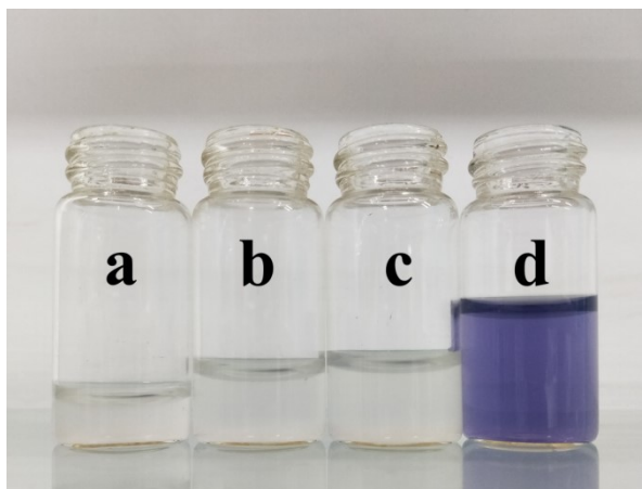
Fig. S4. Detection of \text{H}_2\text{O}_2 . (a) starch+KI; (b) starch+KI+HCl; (c) starch+KI+HCl+molybdate; and (d) starch+KI+HCl+molybdate+supernatant of the reaction mixture.
