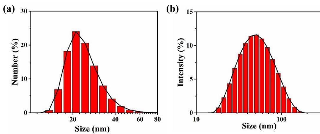
**Figure S4.** DLS size distribution by number (a) and intensity (b) of CM NCs in water.
