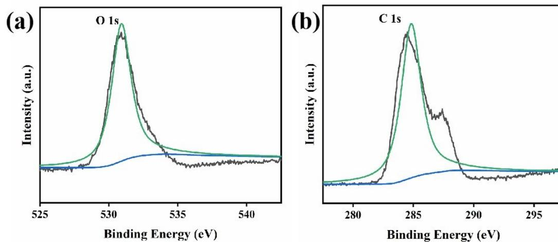
**Figure S2.** XPS survey spectrum of CM NCs. (a, b) O, C element XPS spectra, together with their corresponding fitting curves.
