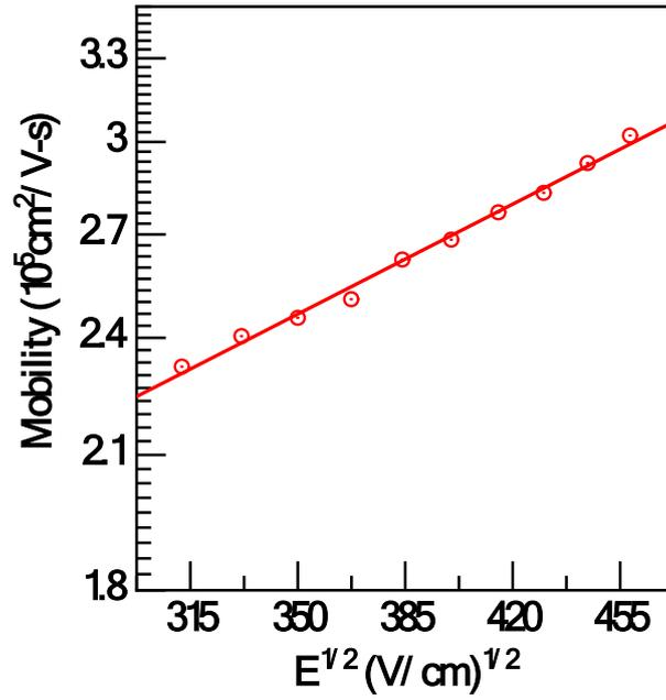
**Figure S5:** Poole-Frenkel (P-F) plot of mobility calculated from the frequency dependent imaginary part of impedance measurement [1] for m-MTDATA based SCL diode. The data fits excellently as a straight line. The y-axis intercept yields the zero-field mobility and the slope corresponds to the P-F coefficient which is found to be  $1.32 \times 10^{-5} \text{ cm}^2 \text{V}^{-1} \text{s}^{-1}$  and  $1.8 \times 10^{-3} \text{ cm}^{1/2} \text{V}^{-1/2}$ , respectively.
