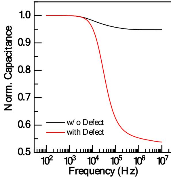
**Figure S4:** Simulated zero bias C-F characteristics with and without defect samples. The Gaussian shape of defect DOS is placed at 0.3eV above the valence band and the holes mobility is considered  $2 \times 10^{-4} \text{ cm}^2\text{V}^{-1}\text{s}^{-1}$  for both cases. Note that the curve is normalized with low frequency capacitance value. Indeed, the defect response is limited by the mobility.
