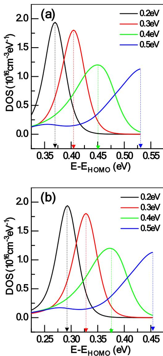
**Figure S7:** Defect DOS distributions extracted from the  $C$ - $f$  curves obtained for varying Gaussian defect level between HOMO and midgap levels. Note that the value of  $\omega_0$  is assumed (a) mobility independent ( $10^{12} \text{s}^{-1}$ ) and (b) mobility dependent. Indeed, the defect level very close to the input defect DOS when the value of  $\omega_0$  is considered mobility dependent.
