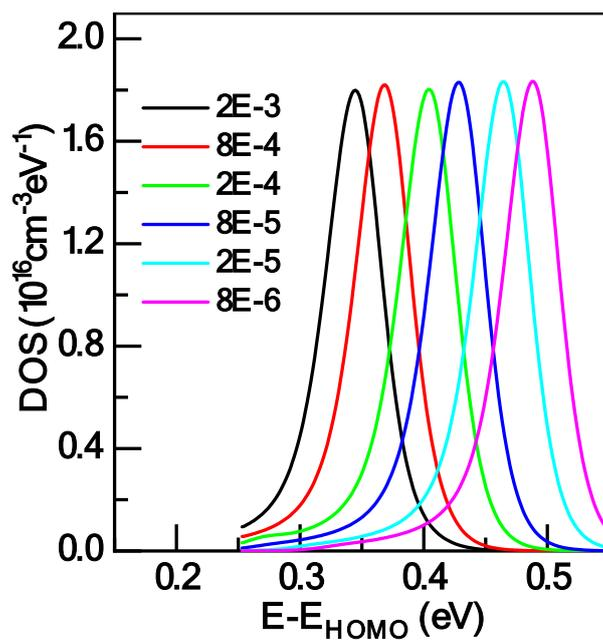
**Figure S6:** Defect DOS distributions extracted from the mobility dependent  $C$ - $f$  curves given in Figure 4 assuming the value of  $\omega_0$  equal to  $10^{12} \text{ s}^{-1}$  [2,3]. Indeed, the defect density does not change with mobility variation, however the peak energy of defect DOS shifts towards the mid of energy gap with decrease of mobility value.
