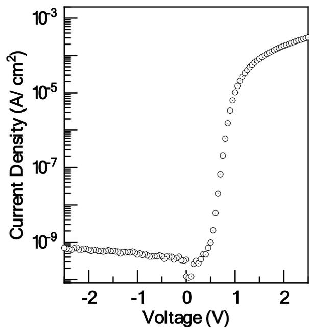
**Figure S2:** Experimental J-V characteristics of 400 nm thick m-MTDATA organic diodes. Note that the rectification ratio is observed more than five orders of magnitudes.
