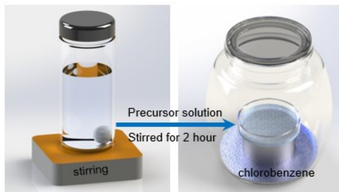
Fig. S1 Schematic illustration of the growth of \text{BA}_2\text{PbBr}_4 single crystal thin films by a gas-liquid interface crystalline route.
