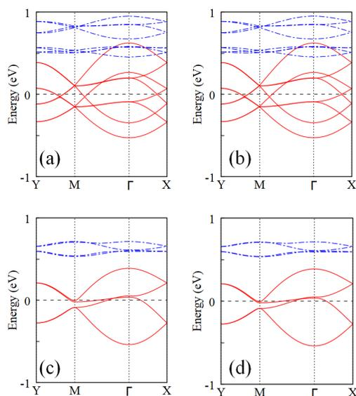
Fig. S1. Band structure of bulk  $\text{CrCl}_2(\text{pyrazine})_2$  calculated by (a) GGA +U and (b) GGA+U+SOC. Band structure of monolayer  $\text{CrCl}_2(\text{pyrazine})_2$  calculated by (c) GGA +U and (d) GGA+U+SOC. The blue (red) lines stand for the up (down) spin. The Fermi level is set at zero energy.
