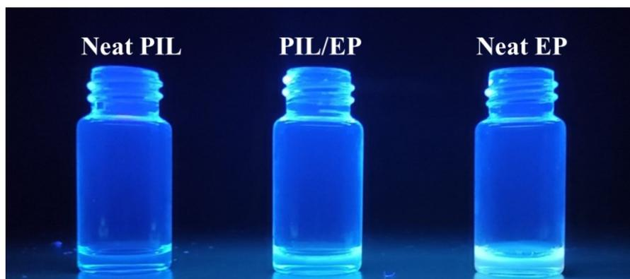
**Fig. S8** Fluorescence images of the neat PIL, PIL/EP, and neat EP (UV light, 365 nm).
