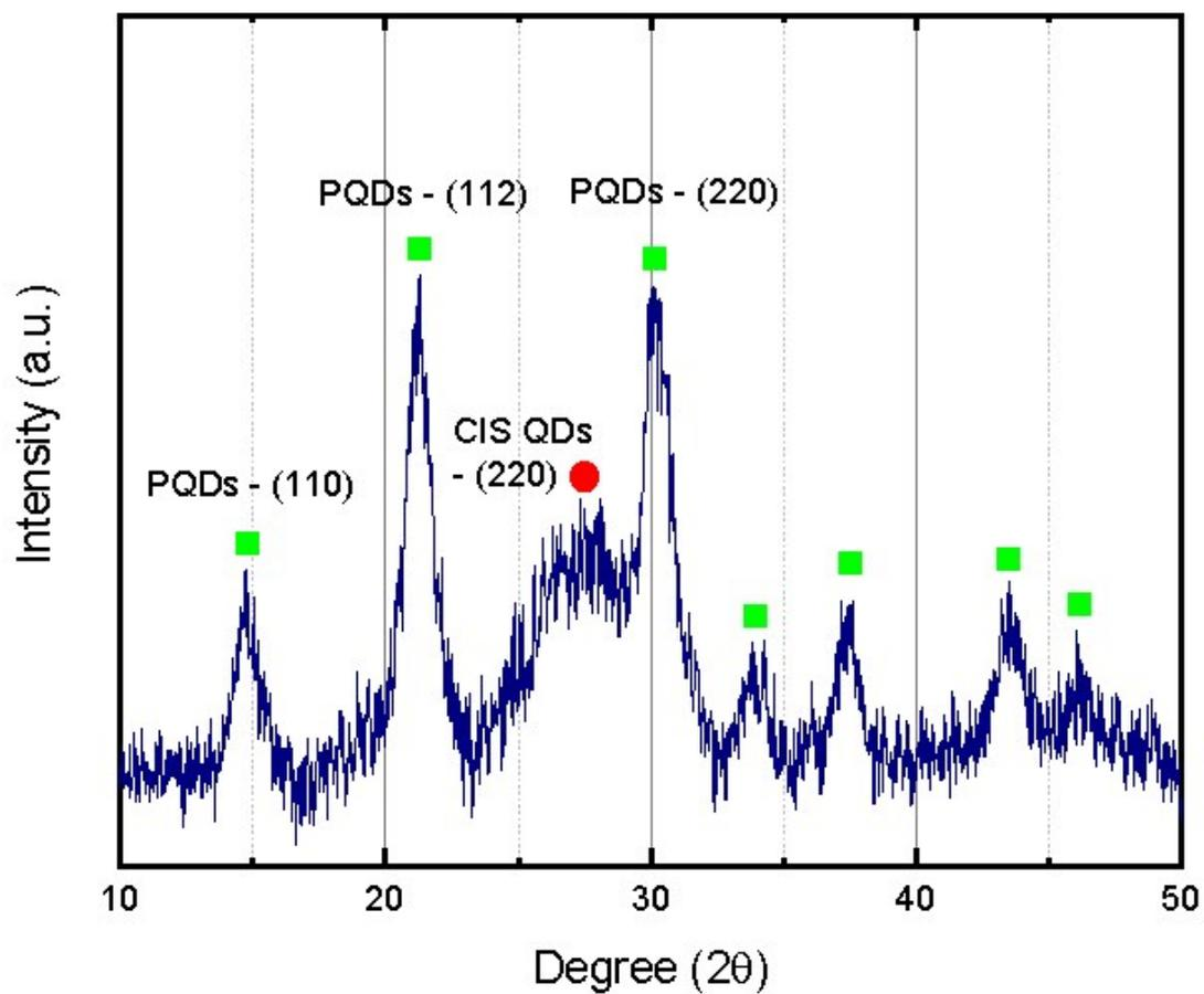
Figure S1. XRD pattern of the mixture of CsPbBr<sub>3</sub> perovskite and CIS quantum composites.
