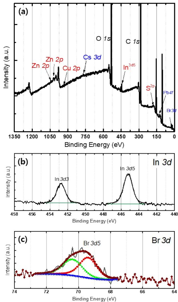
Figure S2. (a) Survey XPS spectra, (b) In 3d peak, and (c) Br 3d peak of the CsPbBr<sub>3</sub> perovskite and CIS quantum composites.
