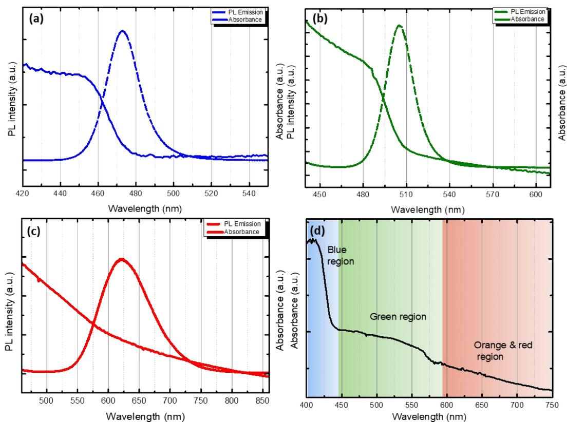
Figure S4. Photoluminescence spectra and UV-vis absorption spectra of (a) blue-emitting, (b) green-emitting perovskite  $\text{CsPb}(\text{Br}_{1-x}\text{Cl}_x)_3$  QDs, and (c) orange-emitting CIS-QDs. (d) UV-vis absorption spectra of property of the perovskite and CIS quantum composites.
