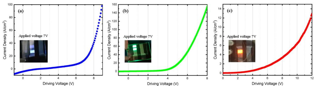
Figure S5. (a) J-V curves of blue-emitting perovskite CsPb(Br<sub>1-x</sub>Cl<sub>x</sub>)<sub>3</sub> QD and (b) green-emitting perovskite CsPbBr<sub>3</sub> QD, and (c) orange-emitting CIS-QDs based LEDs. All emission images of the LED devices were taken at a driving voltage of 7 V.
