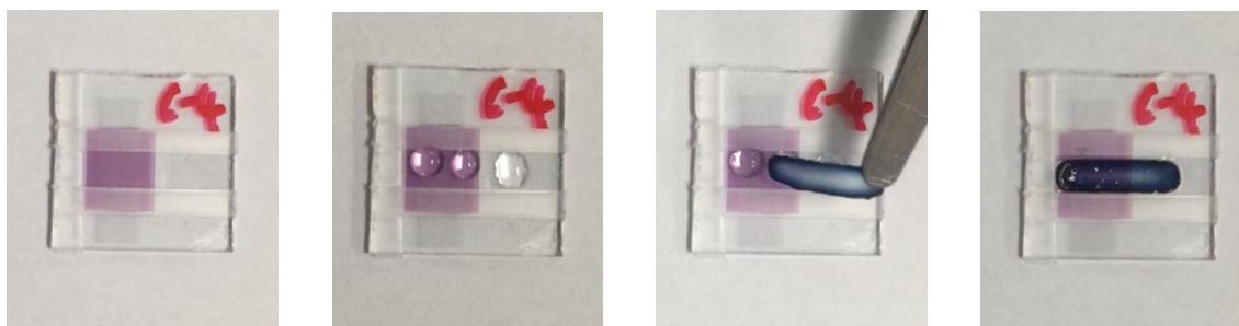
Figure S6 | Adhesion of free standing DVS crosslinked gate electrode using 0.1% GOPS. Photographs show the glass substrate, coated with P3HT and PVP, with strips of tape forming a guide for the gate position. The GOPS solution is then deposited, and the freestanding film is lowered into place.
