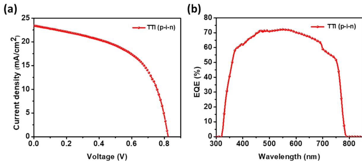
**Figure S6:** Current-voltage ( $J$ - $V$ ) characteristics of inverted structure PSCs based on TTI under Air-Mass (AM) 1.5G illumination and (b) corresponding EQE curve.
