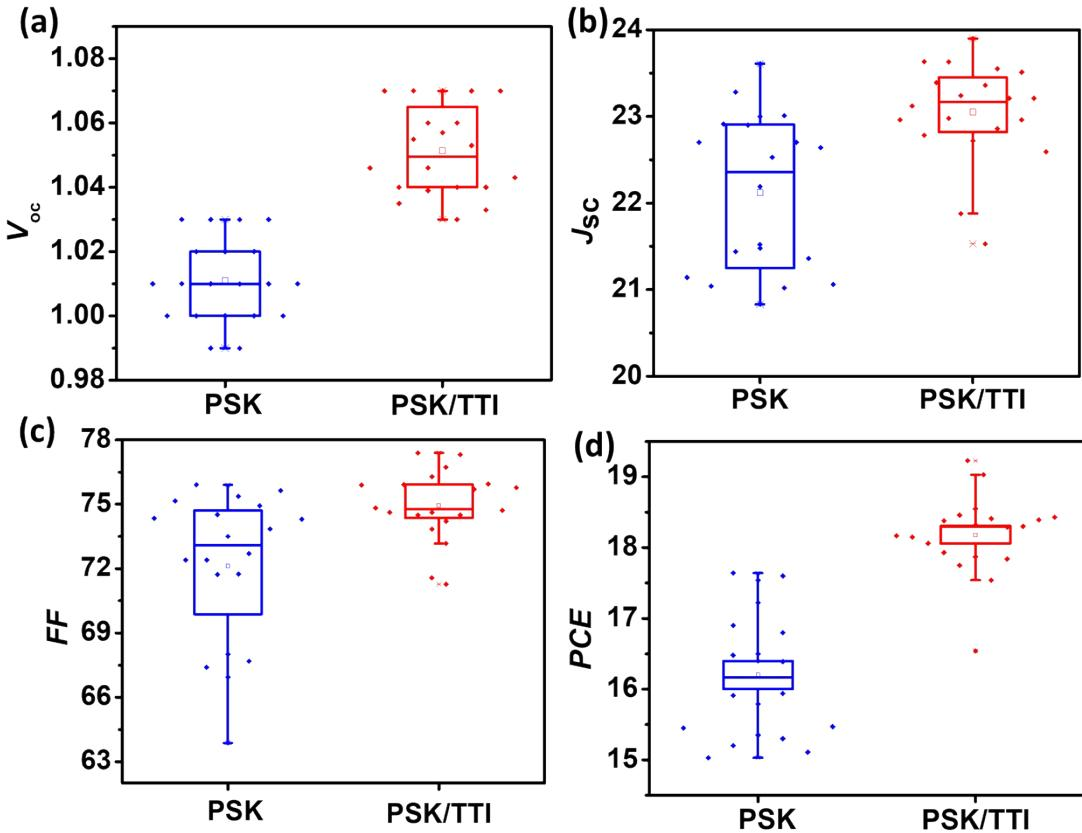
**Figure S9:** Device statistics (20 devices each) (a)  $V_{oc}$ , (b)  $J_{sc}$ , (c) FF and (d) PCE, for pristine {PSK} and passivated (PSK/TTI) PSCs.
