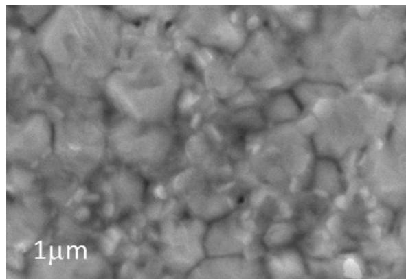
**Figure S5:** Surface SEM image of perovskite and TTI as the HTM layer.
