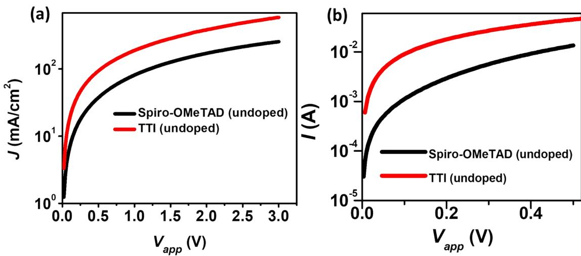
**Figure S3:** (a) Hole mobility measurements (device structure: FTO/PEDOT: PSS/HTM/Au) and (b) conductivity measurements (device structure: FTO/HTM/Au); of the undoped TTI and Spiro/OMeTAD.
