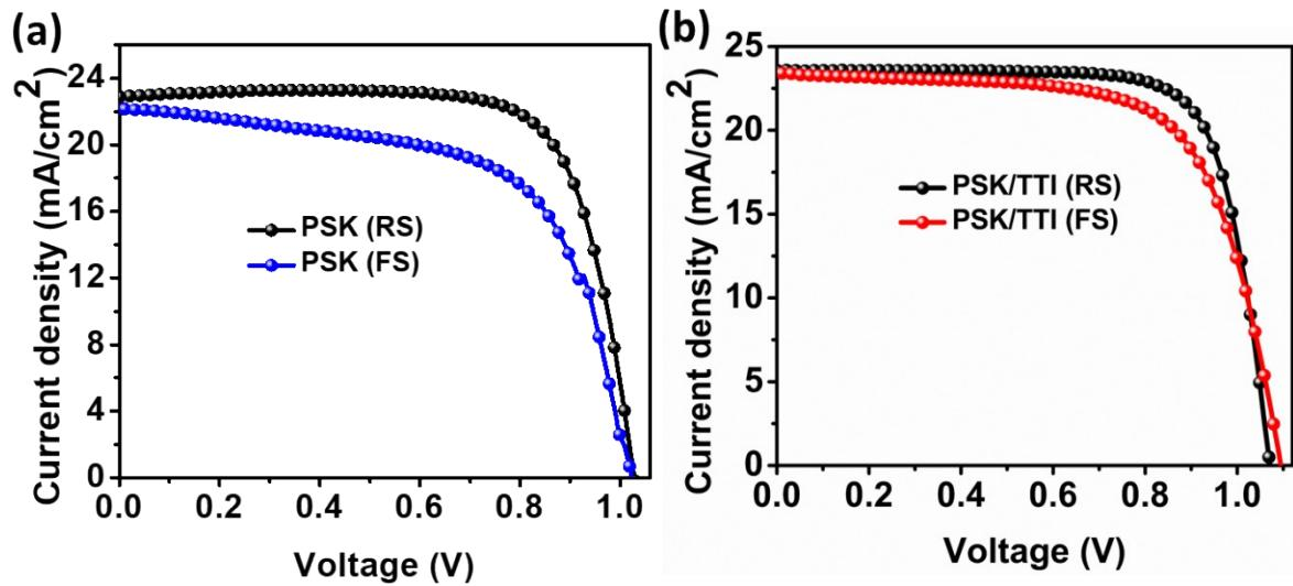
**Figure S8:**  $J$ - $V$  characteristic of forward scan and reverse scan for (a) pristine {PSK} and (b) TTI passivated PSCs.
