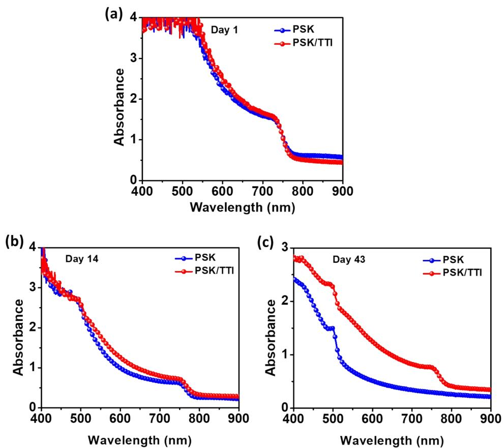
**Figure S11:** Absorption spectra of pristine perovskites (PSK) and PSK/TTI passivated perovskites under thermal annealing at 85°C (a) Day 1 (b) Day 14 and (c) Day 43.
