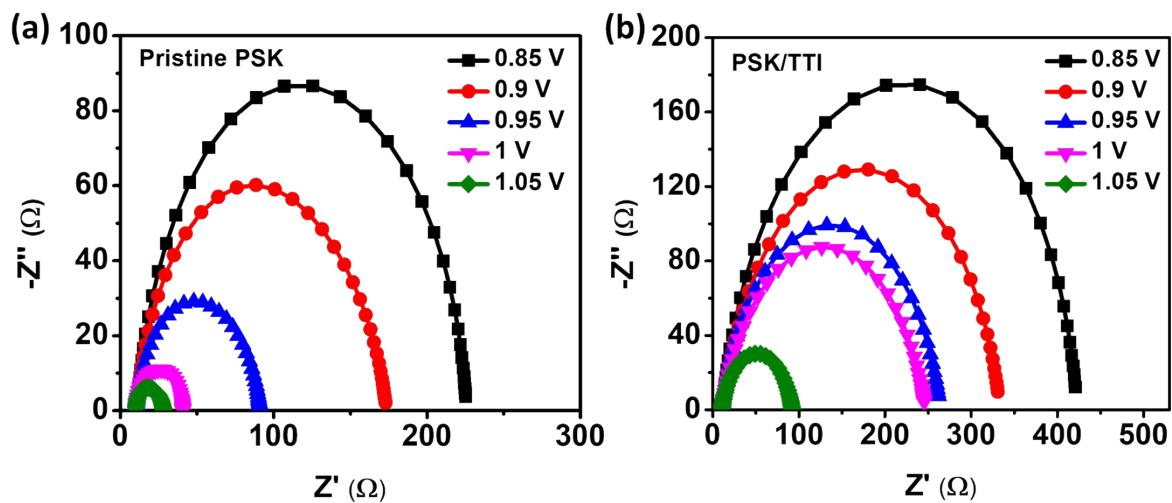
**Figure S10:** Nyquist plots for PSC, (a) pristine and (b) TTI passivated at variable voltages.
