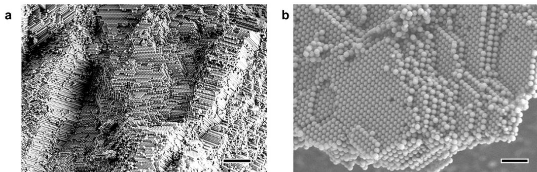
**Fig. S13** SEM images of the SiO<sub>2</sub> part from a broken supraparticle. Scale bars are 5 μm for (a) and 1 μm for (b).
