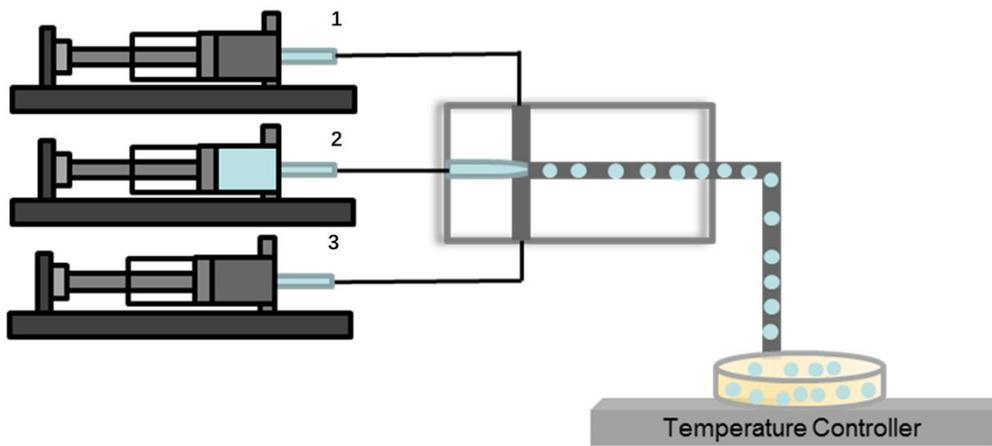
**Fig. S8** The microfluidic device for the generation of droplets.
