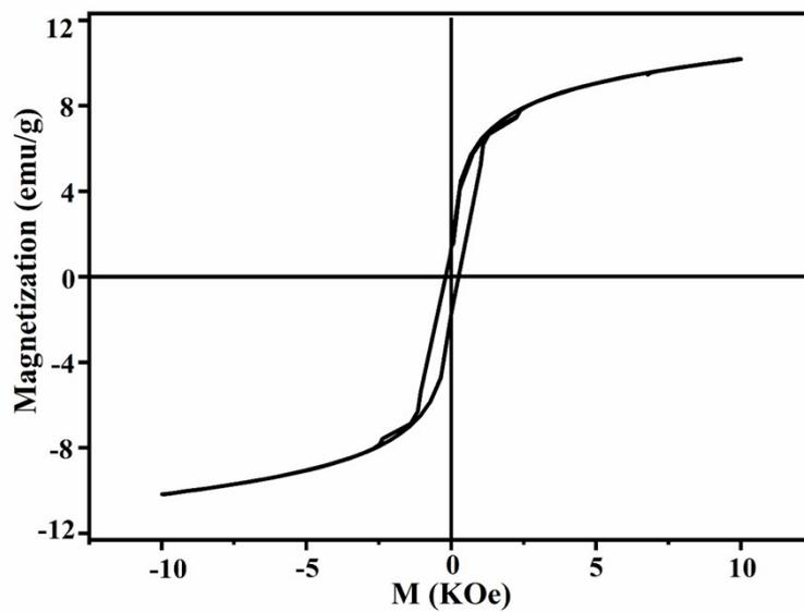
**Fig. S6** Hysteresis loop of the  $\text{Fe}_3\text{O}_4@\text{SiO}_2$  nanoellipsoids at room temperature.
