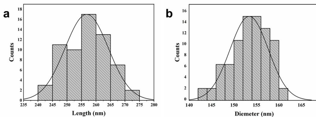
**Fig. S4** Size distribution of  $\text{Fe}_3\text{O}_4@\text{SiO}_2$  nanoellipsoids. (a) Their average length, obtained by measuring 100 particles, is  $255 \pm 10$  nm. (b) Their average diameter, obtained by measuring the same 100 particles, is  $155 \pm 5$  nm.
