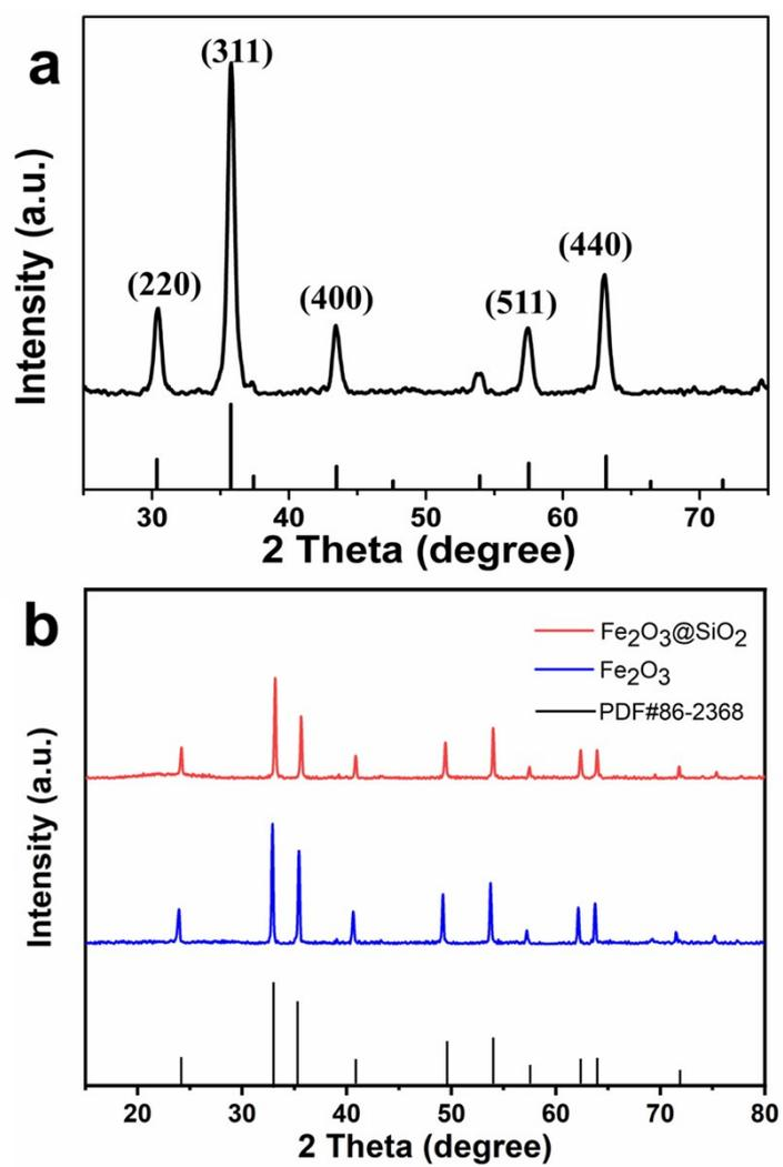
**Fig. S2** XRD patterns of (a)  $\text{Fe}_3\text{O}_4@SiO_2$ , and (b)  $\alpha\text{-Fe}_2\text{O}_3$  and  $\alpha\text{-Fe}_2\text{O}_3@SiO_2$  nanoellipsoids.
