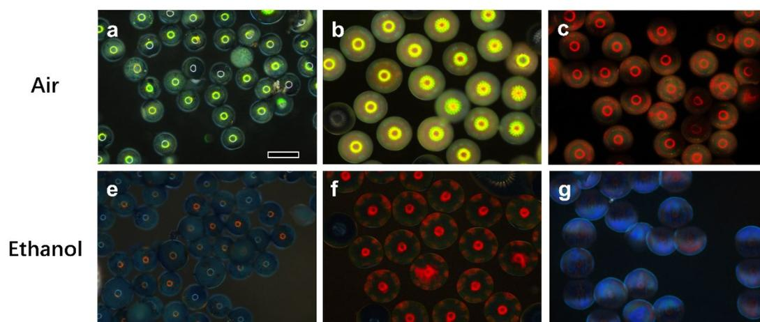
**Fig. S15** Dark-field optical microscope images of supraparticles made up of different sizes SiO<sub>2</sub>. Scale bar is 100  $\mu\text{m}$ .
