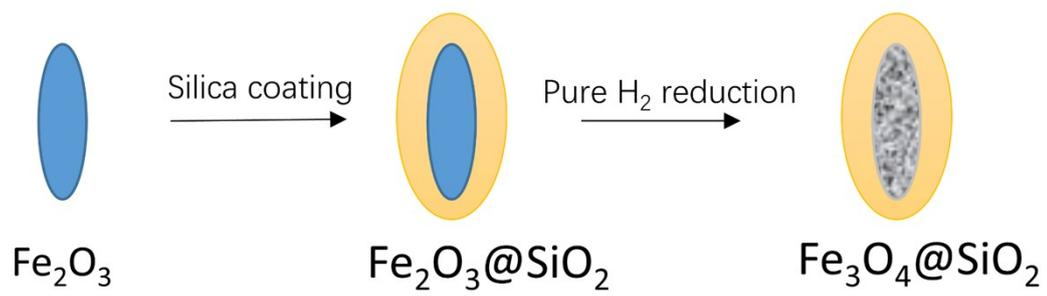
**Fig. S1 Schematic illustration of the preparation process of Fe<sub>3</sub>O<sub>4</sub>@SiO<sub>2</sub> nanoellipsoids.**
