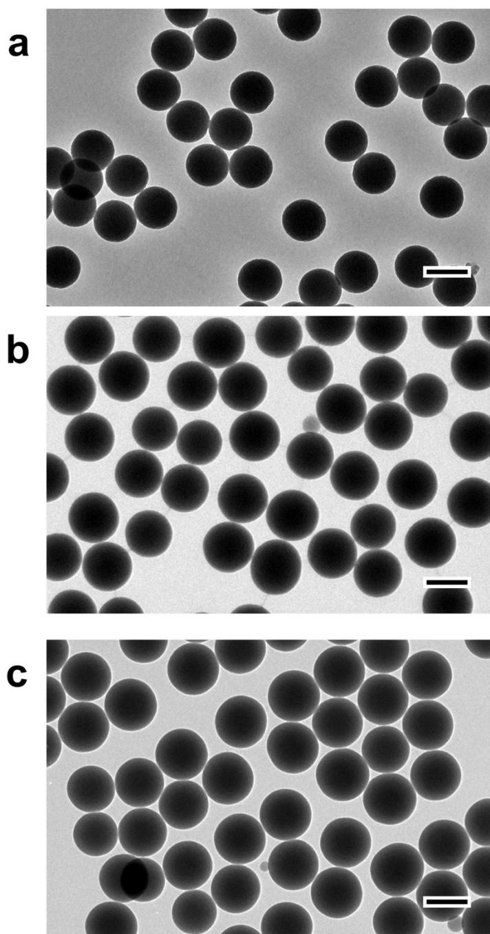
**Fig. S7** TEM images of SiO<sub>2</sub> nanospheres of different sizes: (a) 220 nm, (b) 260 nm, (c) 300 nm. Scale bars are 200 nm.
