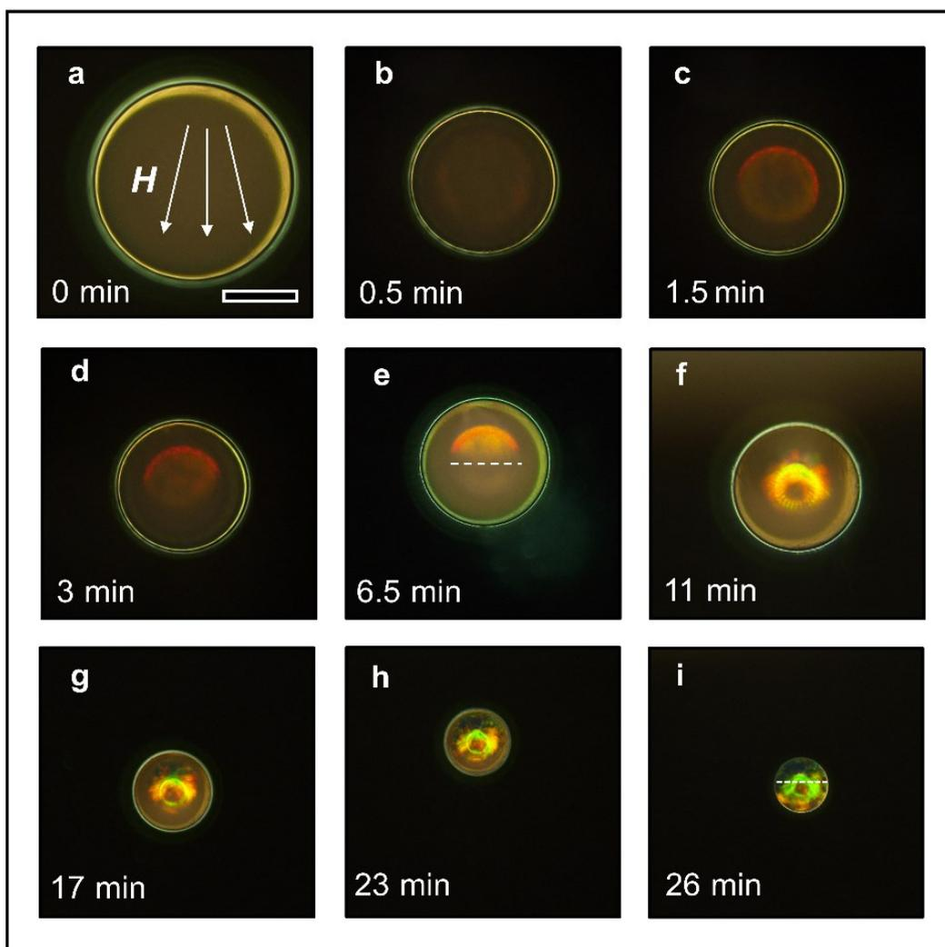
**Fig. S9** Optical microscopy images showing the assembly process of a single droplet under the horizontal magnetic field. Scale bar is 100  $\mu\text{m}$ .
