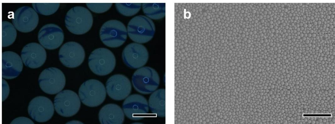
**Fig. S14** (a) Optical microscopy and (b) SEM images of supraparticles dried in the absence of magnetic fields. Scale bars are 100  $\mu\text{m}$  for (a) and 1  $\mu\text{m}$  for (b).
