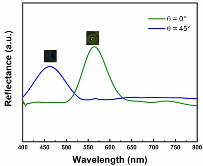
**Fig. S16** Reflection spectra of supraparticles in response to magnetic fields with different directions.
