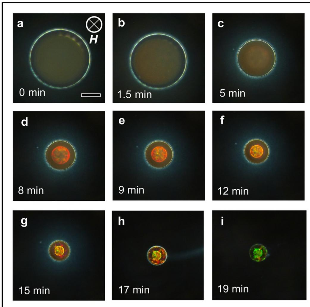
**Fig. S10** Optical microscopy images showing the assembly process of a single droplet under the vertical magnetic field. The field strength decreased from the bottom to the top. Scale bar is 100  $\mu\text{m}$ .
