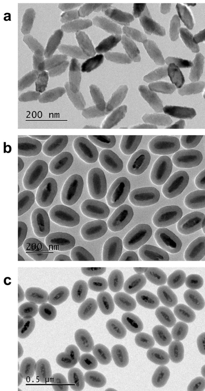
**Fig. S3** TEM images of (a)  $\alpha$ - $\text{Fe}_2\text{O}_3$ , (b)  $\alpha$ - $\text{Fe}_2\text{O}_3$ @ $\text{SiO}_2$  and (c)  $\text{Fe}_3\text{O}_4$ @ $\text{SiO}_2$  nanoellipsoids.
