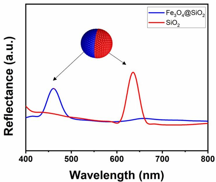
**Fig. S11** Reflection spectra of the two parts of a supraparticle.
