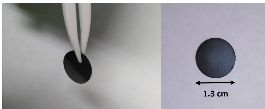
Fig. S3: The pressed thick films were obtained by pressing 0.4 g of the dry perovskite powder with 100 MPa on a homemade mechanical press. The diameter of the free-standing pellets is 1.3 cm and the thickness is about 0.8 mm. The density of the pellets therefore is about (3.75 \pm 0.05) \text{ g/cm}^3 .
