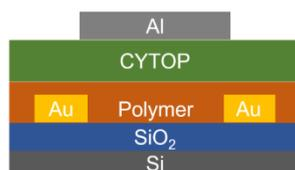
**Figure S11.** The TG/BC OFET device architecture.
