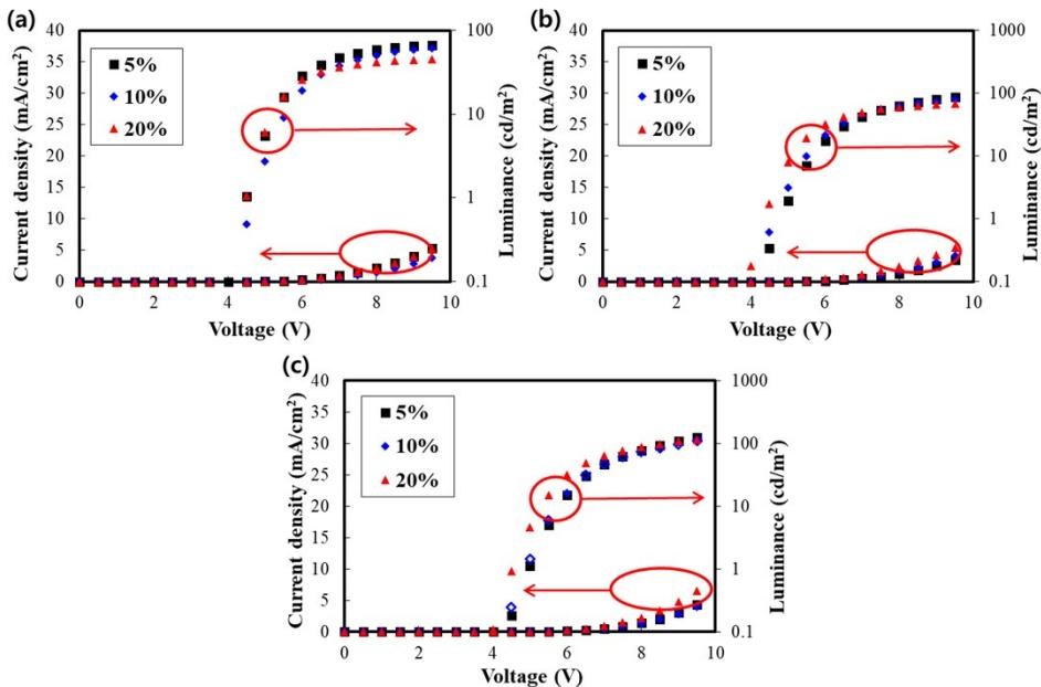
**Figure S6.** The data of current density and luminance according to driving voltage. ((a) PhSe, (b) mPhSe, and (c) BuPhSe.)
