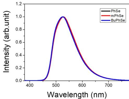
**Figure S5.** The EL spectra of the purely organic based PhOLEDs at doping concentration of 20 wt%.
