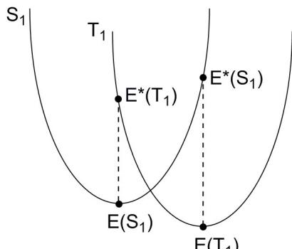
$$\lambda_M (S_1 \rightarrow T_1) = E^*(T_1) - E(T_1)$$
