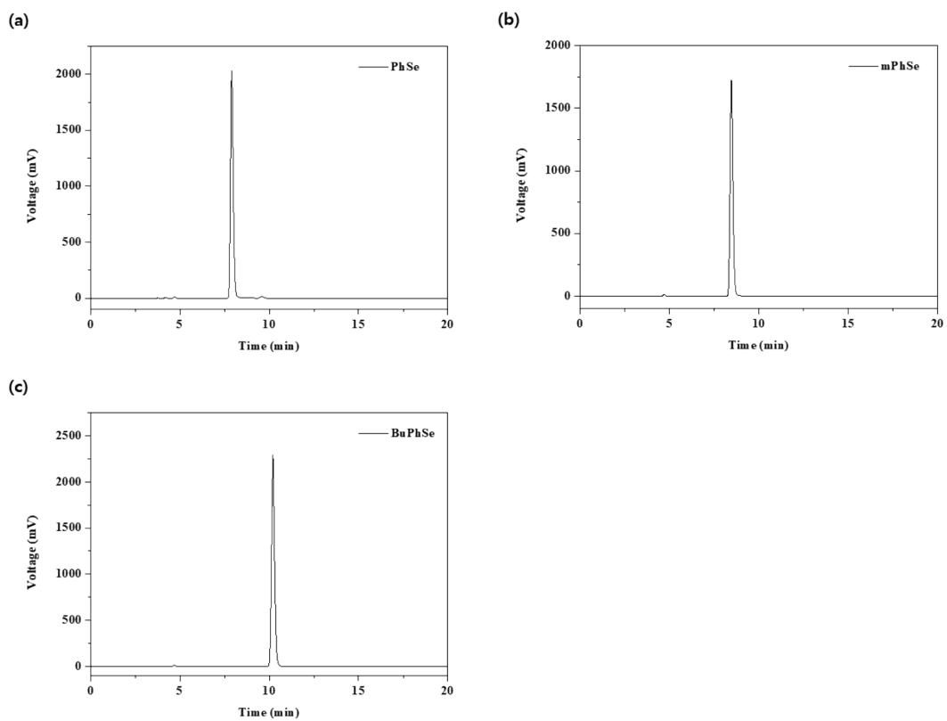
**Figure S3.** HPLC spectra of PhSe (a), mPhSe (b), and BuPhSe (c).
