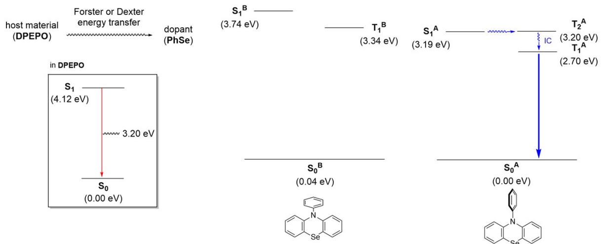
**Figure S8.** Jablonski diagram of  $\text{PhSe}_A$ ,  $\text{PhSe}_B$ , and DPEPO host material
