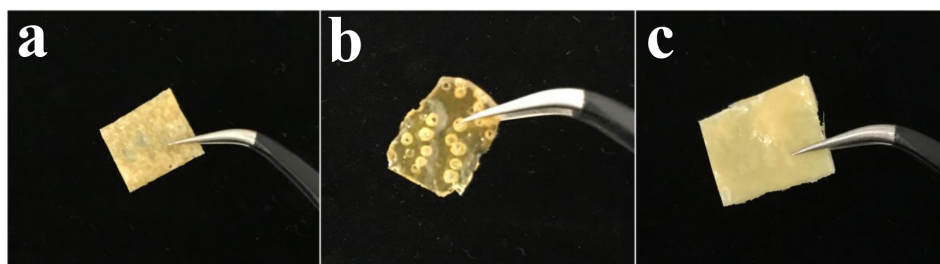
Fig. S4 Poly(ionic liquid) films of [\text{C}_4\text{VIM}]\text{Mn}_1 (a), [\text{C}_8\text{VIM}]\text{Mn}_2 (b) and [\text{C}_{12}\text{VIM}]\text{Mn}_3 (c).
