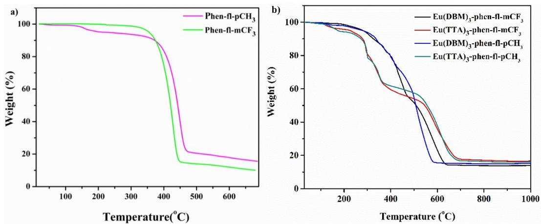
Fig. S5. TGA of ligand (a) and  $\text{Eu}(\text{III})$  complexes (b).
