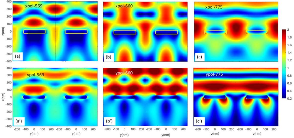
**Fig. S2.** Mode field enhancement profiles for the structure shown in Fig. 6c, corresponding to sample 3, in the y-z plane at wavelengths 569, 660, and 775 nm for  $\theta_i=0^\circ$  (a-c) and  $\theta_i=90^\circ$  (a'-c'). Here the refractive index of the superstrate is considered to be 1.33.
