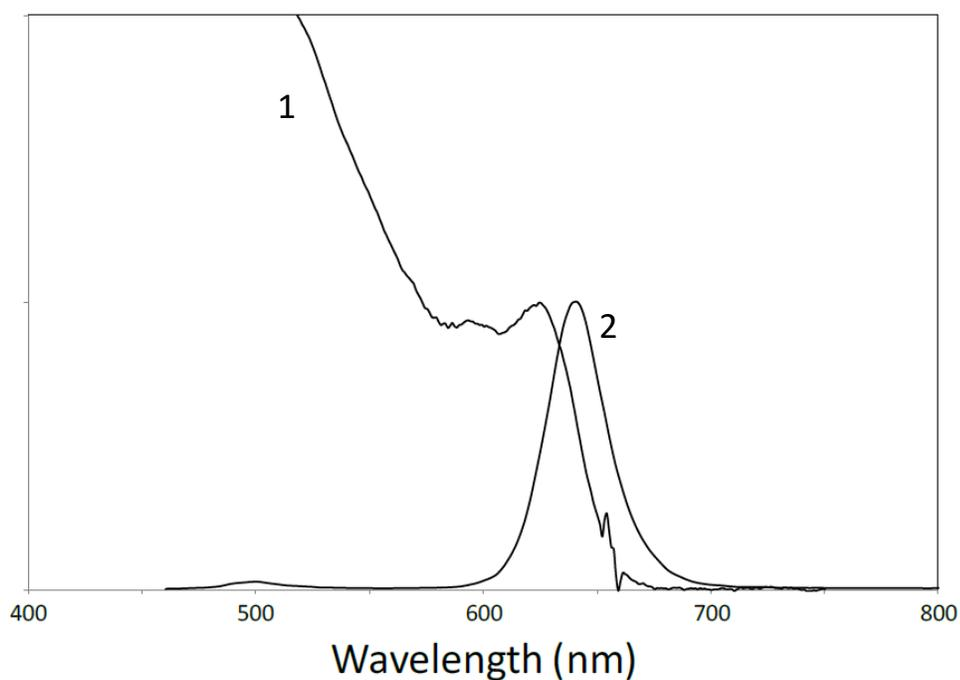
**Fig. S1.** Absorption (line 1) and emission spectra (line 2) of QDs as provided by NNCrystal US Corporation (NN Labs LLC).
