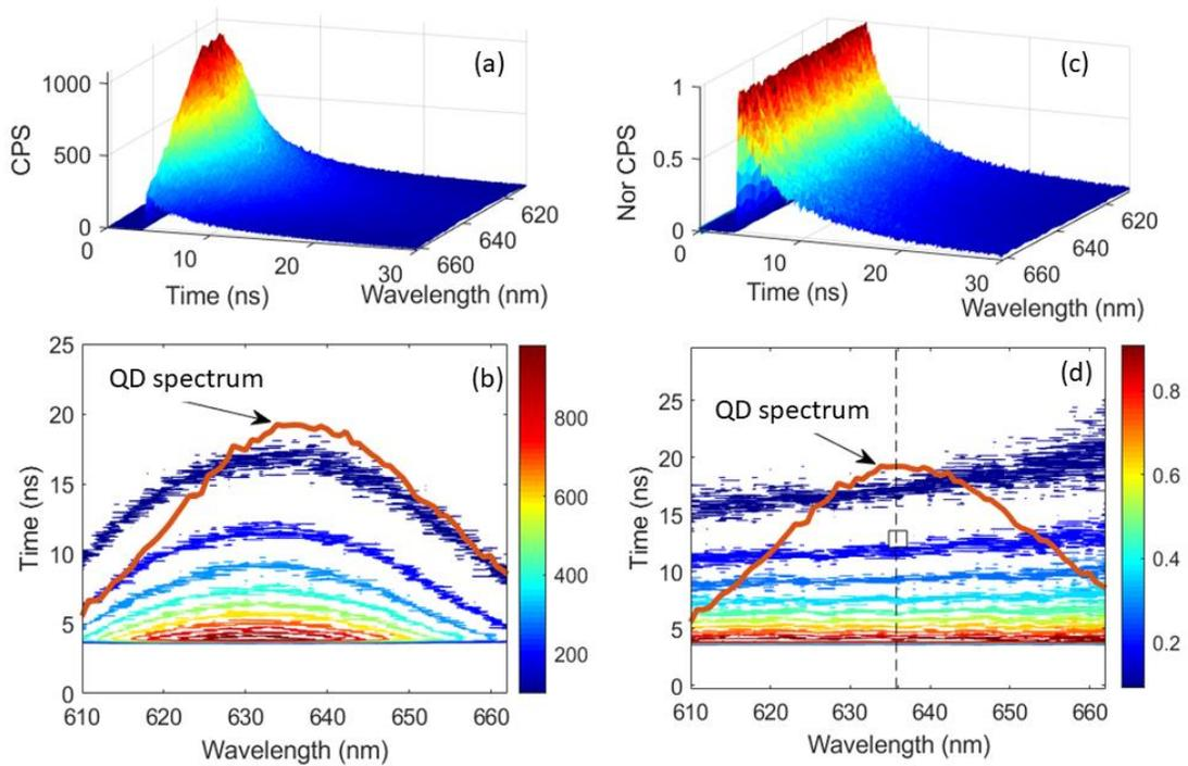
**Fig. S3.** Wavelength-resolved decay of QDs on sample 3 (a) and its contour (b). (c) the normalized decay shown in (a), and (d) presents its contour. CPS refers to counts per second. The thick red lines in (b) and (d) show the emission spectrum of the QDs in the wavelength range shown in these figures.
