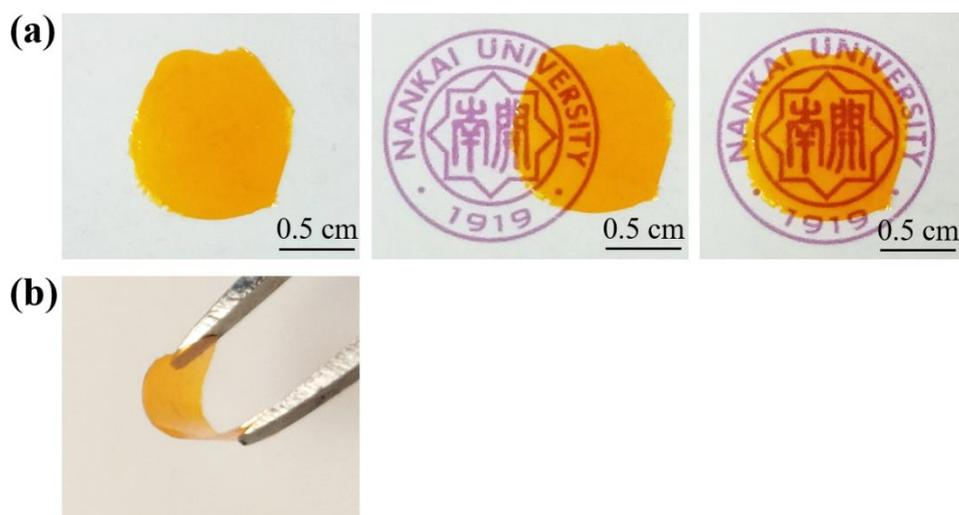
**Fig. S4** Photographs of a free-standing PEU-10 film (prepared via the special melt pressing method) that is transparent (a) and flexible (b) at room temperature.
