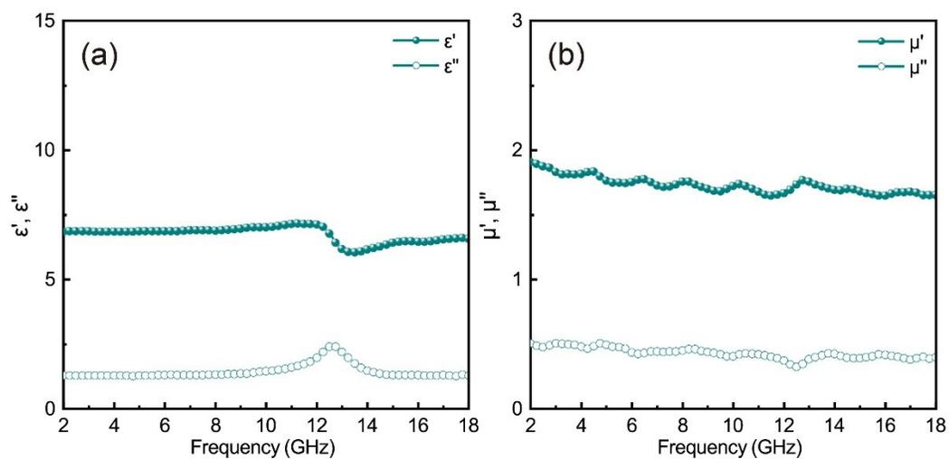
**Fig. S6** Electromagnetic parameters of FeCoNi NSs. (a) the real/imaginary parts of complex permittivity; (b) the real/imaginary parts of complex permeability.
