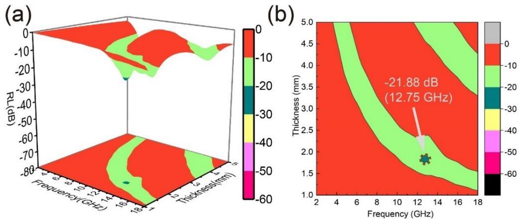
**Fig. S5** 3D/2D RL contour maps of FeCoNi NSs.
