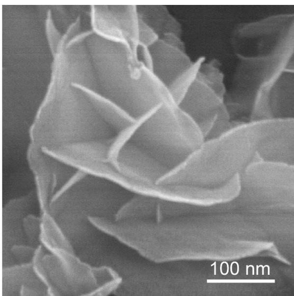
**Fig. S1** SEM image of FeCoNi NSs
