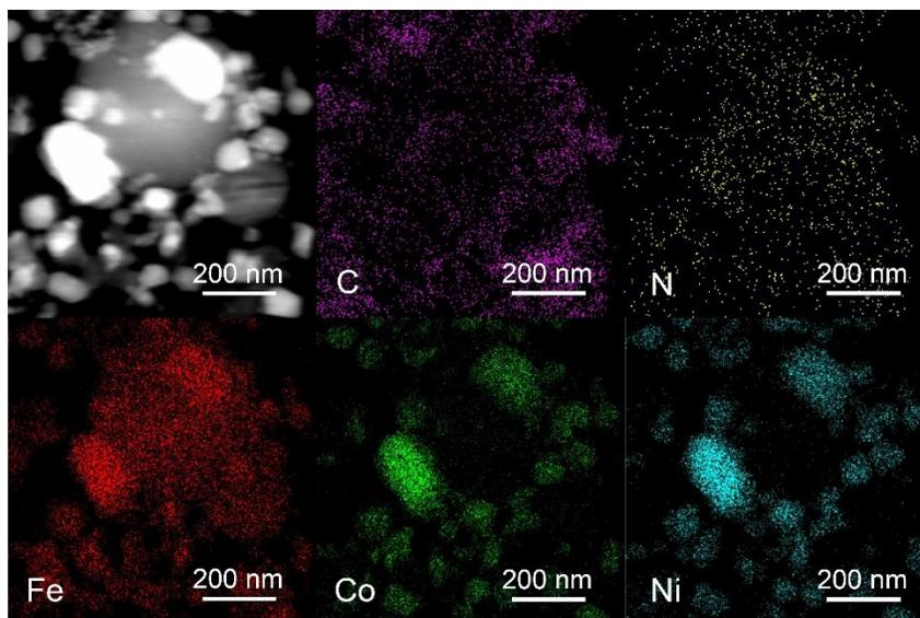
**Fig. S2** HAADF-STEM and elemental mapping of FeCoNi@HC composites at 900 °C
