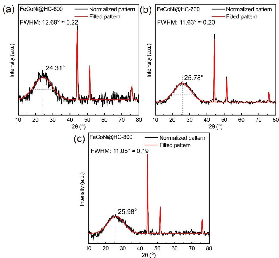
**Fig. S3** Normalized XRD patterns for confirming  $\theta$  and  $\beta$  values based on the (002) peaks
