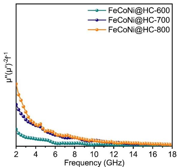
Fig. S7  $C_0$  curves of the FeCoNi@HC composites
