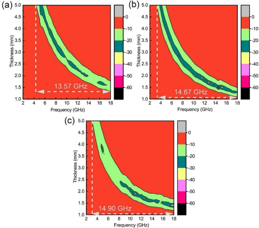
**Fig. S4** 2D RL contour maps of the FeCoNi@HC composites. (a) FeCoNi@HC-600; (b) FeCoNi@HC-700; (c) FeCoNi@HC-800.
