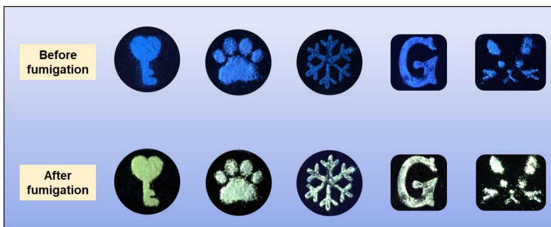
Figure S20 Luminous images of different templates filled with PTZ-3Cl-eq before and after DCM fumigation under UV irradiation at 365 nm.
