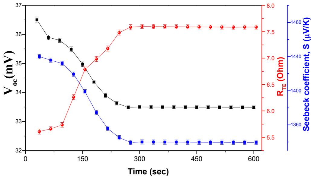
Figure S2. Thermoelectrical properties over time for the 28 days cement/SWCNT(0.5) sample over 10 minutes.
