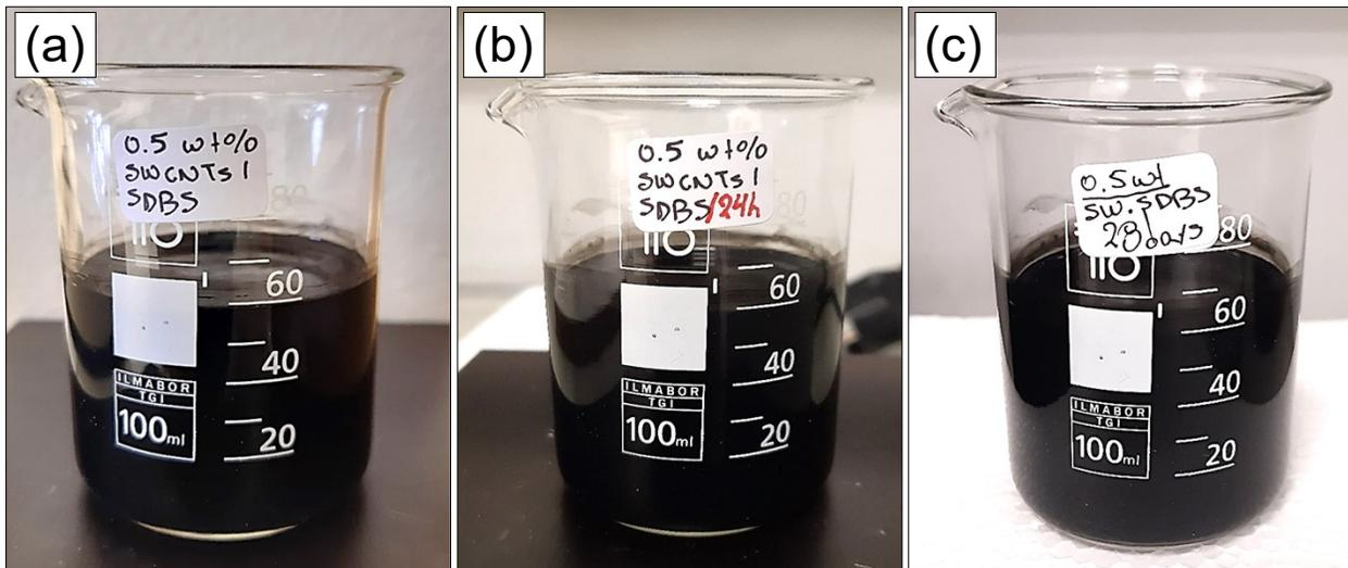
Figure S1. SWCNT dispersions (a) immediately after ultrasonication, (b) after  $t = 24$  hours, and (c) after  $t = 28$  days, without any observed aggregates and sedimentation by time.
