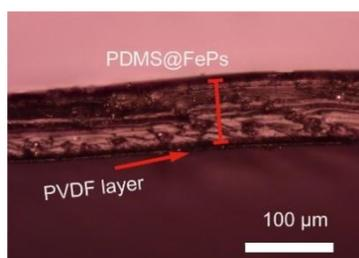
**Fig. S5** The microscopic image of the cross section of a bilayer of PVDF/PDMS@FePs.
