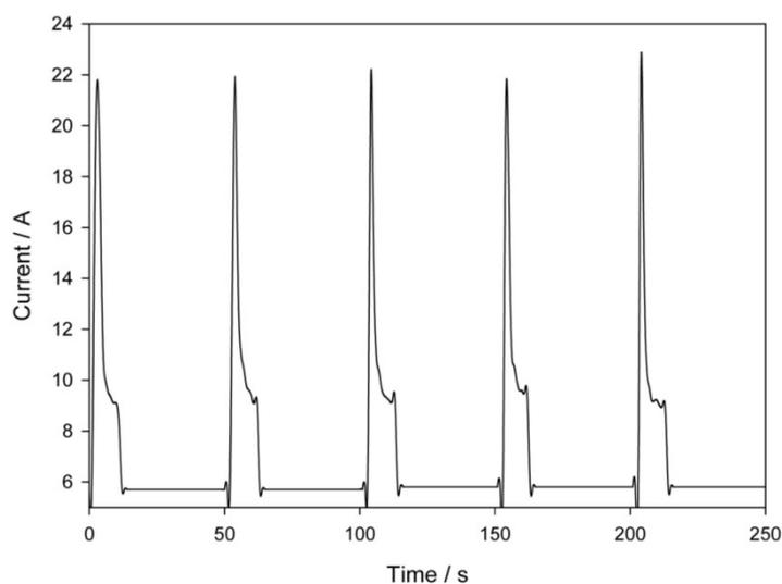
**Fig. S7** The profile recording the current change passing through the energized coil at a high power mode (400 W).
