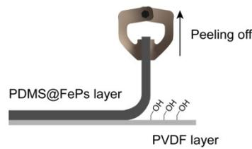
**Fig. S3** Sketch map showing how to do a standard 90° peeling test for the bilayer. The result was used to evaluate the interfacial stability during the actuation by magnetocaloric effects.
