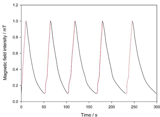
**Fig. S6** The magnetic field intensity variation caused by a rectangular sheet iron. As the sheet iron was inserted into the induction coil, the intensity of magnetic field was increased greatly; while it was retracted, the intensity of magnetic field decreased.
