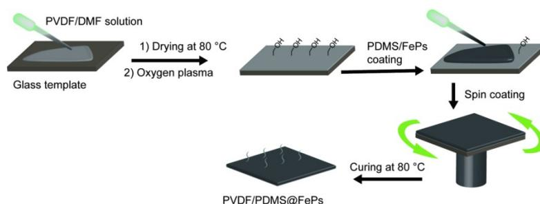
**Fig. S1** The manufacturing process of the PVDF/PDMS@FePs bilayer actuators.
