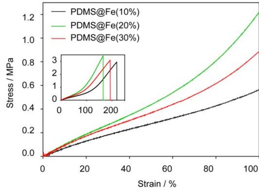
**Fig. S2** Mechanical tests of the PDMS@FePs single layer with different FePs content to figure out the FePs content effects on the stiffness of the bilayer.
