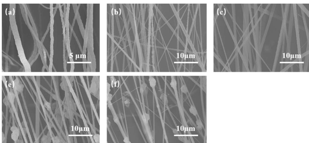
Fig. S1 The SEM photos of the aligned nanofibers prepared from spinning solutions with different PVP mass fractions of 3.8%(a), 3.9%(b), 4.3%(c), 4.6%(d) and 5.0%(e).
