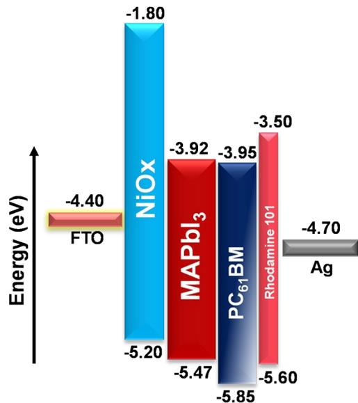
**Fig. S1** Energy band diagram of constituent layers in PVSC.
