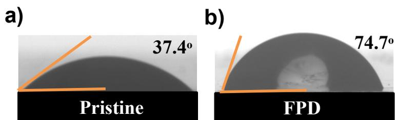
Fig. S4 Contact angle of a) pristine and b) FPD passivated films.
