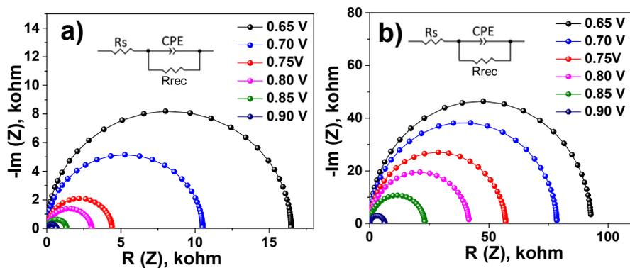
**Fig. S2** Nyquist plots obtained from impedance spectroscopy conducted at varied bias (0.65 V - 0.90 V) for a) pristine b) FDP passivated PVSCs.
