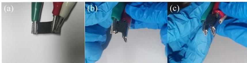
Fig. S4 Photographs of the devices at various bending states. (a)  $0^\circ$ ; (b)  $90^\circ$ ; (c)  $180^\circ$ .
