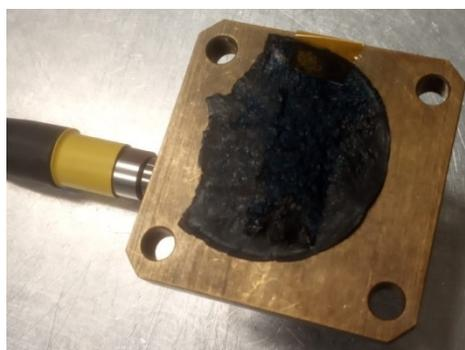
**Fig. S1** The rectangular opening of the WR 90 waveguide (22.86 mm × 10.16 mm) completely covered with PEDOT:PSS hydrogel film.
