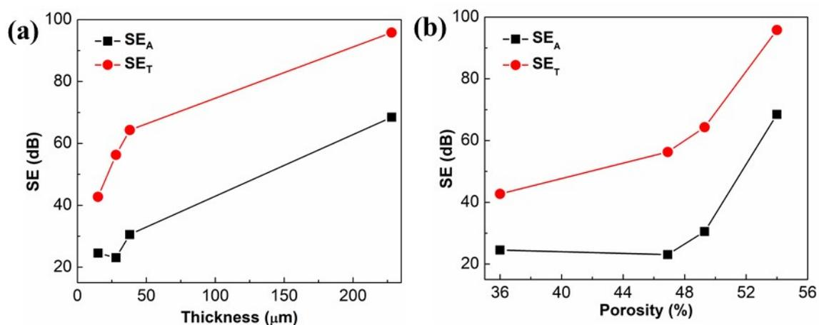
**Fig. S11:** (a-b) Variation of SE<sub>A</sub> and SE<sub>T</sub> as a function of thickness and porosity for PEDOT:PSS hydrogel films. Note, SE values are taken at a representative frequency value of 9 GHz.
