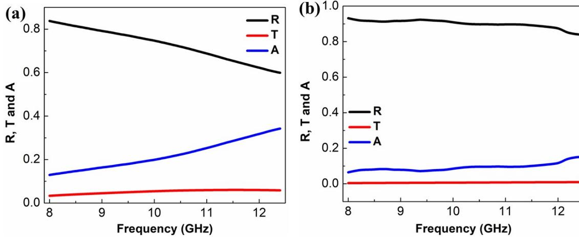
**Fig. S9:** (a-b) Variation of R, T and A as a function of frequency for uncompressed and compressed PEDOT:PSS sponges.
