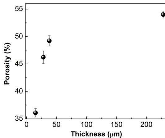
**Fig. S5:** Variation of porosity as a function of PEDOT:PSS hydrogel film thickness.
