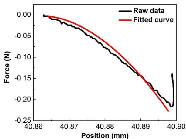
**Fig. S3** Force versus position plot (indentation test). 0.5 mm diameter spherical indenter attached to a load cell was indented on the hydrogel film to estimate the Young's modulus. Black and red solid line represent raw data and fitted curve, respectively.
