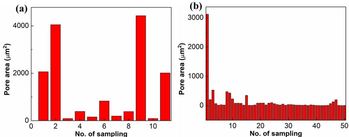
**Fig. S6:** (a-b) Bar plot of pore area as a function of number of sampling for uncompressed and compressed PEDOT:PSS sponge.
