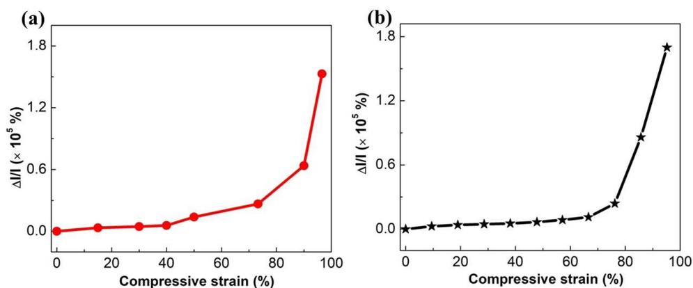
**Fig. S4** (a-b) Variation of normalized current as a function of strain under unconfined compression for PEDOT:PSS sponge (sample 2 and sample 3).
