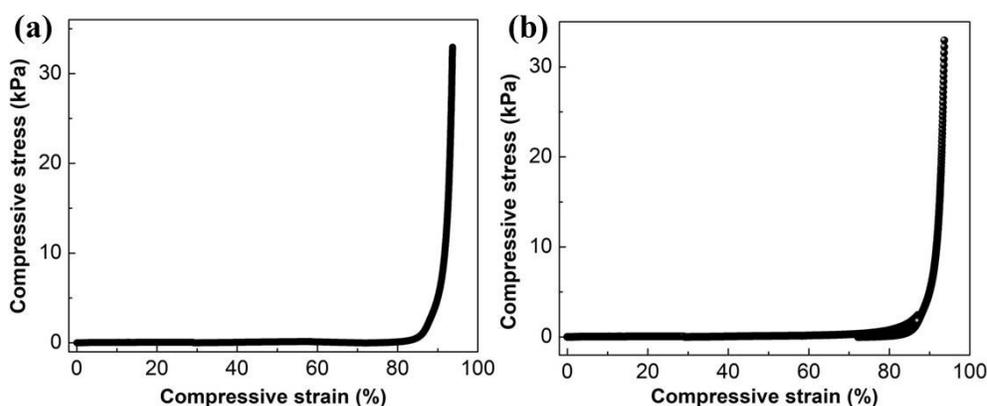
**Fig. S2** (a-b) Compressive stress-strain curve of PEDOT:PSS sponge (sample 2 and sample 3).
