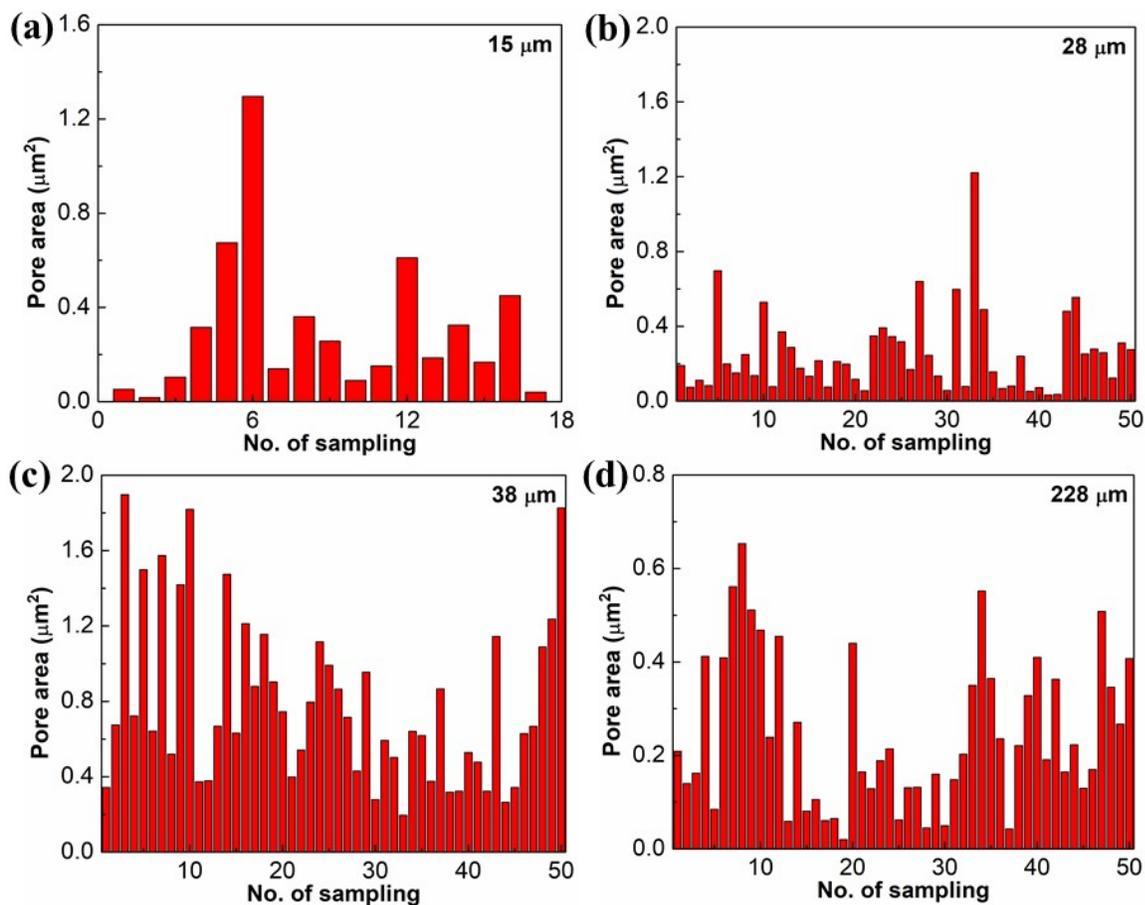
**Fig. S7:** (a-d) Bar plot of pore area as a function of number of sampling for 15  $\mu\text{m}$ , 28  $\mu\text{m}$ , 38  $\mu\text{m}$  and 228  $\mu\text{m}$  thick PEDOT:PSS hydrogel film.
