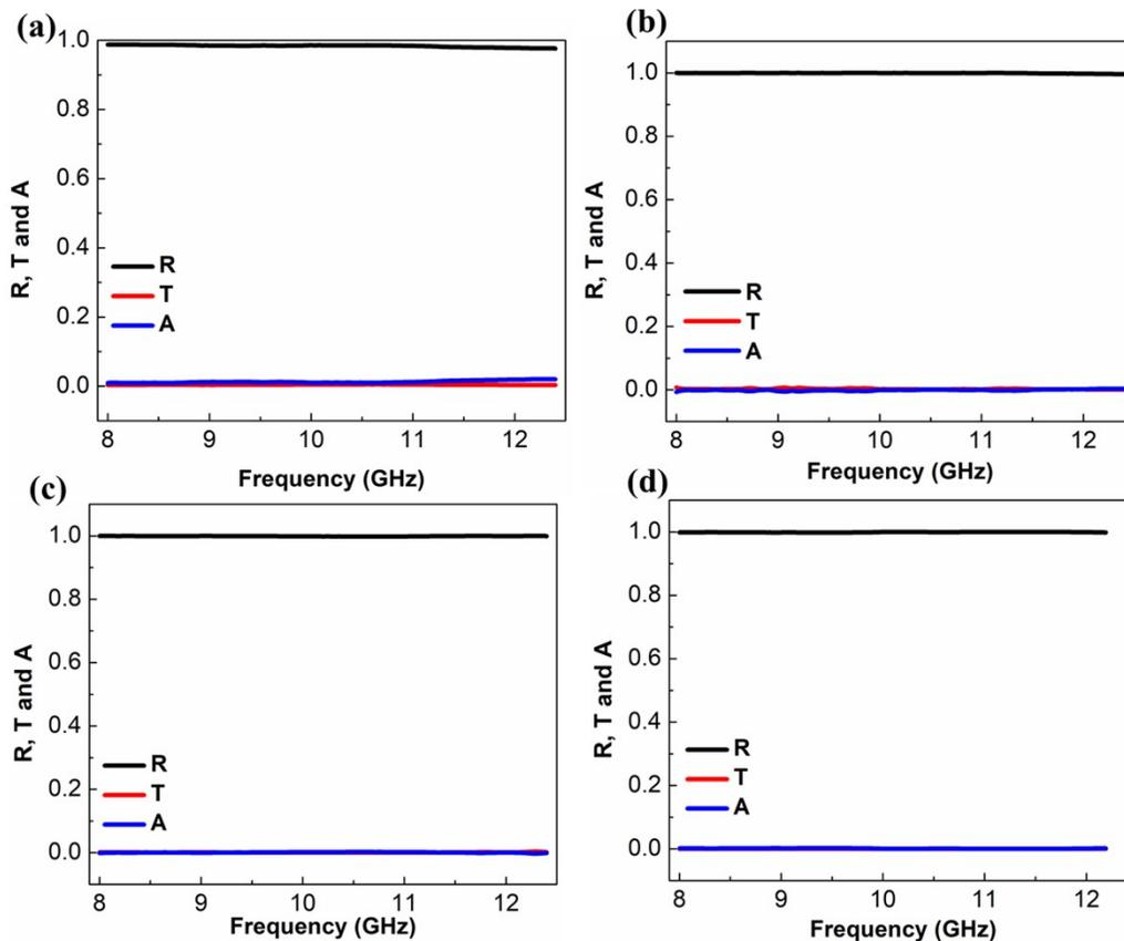
**Fig. S10:** (a-d) Variation of R, T and A as a function of frequency for 15  $\mu\text{m}$ , 28  $\mu\text{m}$ , 38  $\mu\text{m}$  and 228  $\mu\text{m}$  thick PEDOT:PSS hydrogel film.
