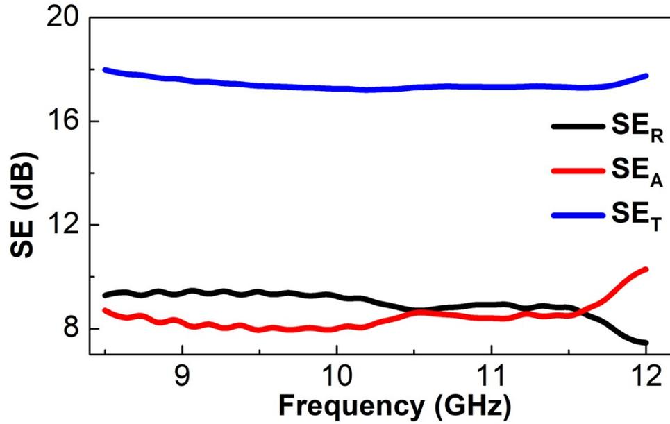
Fig. S8: Variation of EMI SE as a function of frequency for a pure PEDOT:PSS film.
