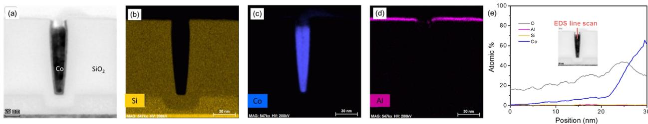
**Figure S3.** FC10PA-treated Co/SiO<sub>2</sub> patterned substrate consisting of 20 nm wide Co-filled SiO<sub>2</sub> trenches after 10 cycles of Al<sub>2</sub>O<sub>3</sub> ALD: (a) bright-field cross-sectional TEM image, (b-d) EDS composition mapping analysis of Si, Co, and Al elements (yellow, blue, and pink colors), and (e) cross-sectional TEM line scans. The TEM line scan direction is marked by the red line.
