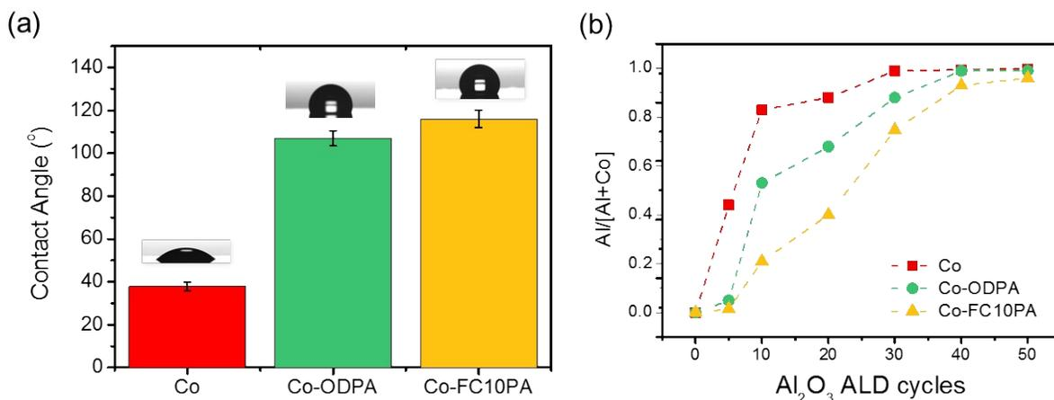
**Figure S1.** (a) Contact angles measurements of water on the surfaces of untreated, ODPA-modified, and FC10PA-modified Co substrates. (b) XPS composition analysis on the surfaces of Co, Co-ODPA, and Co-FC10PA after different cycles of Al<sub>2</sub>O<sub>3</sub> ALD.
