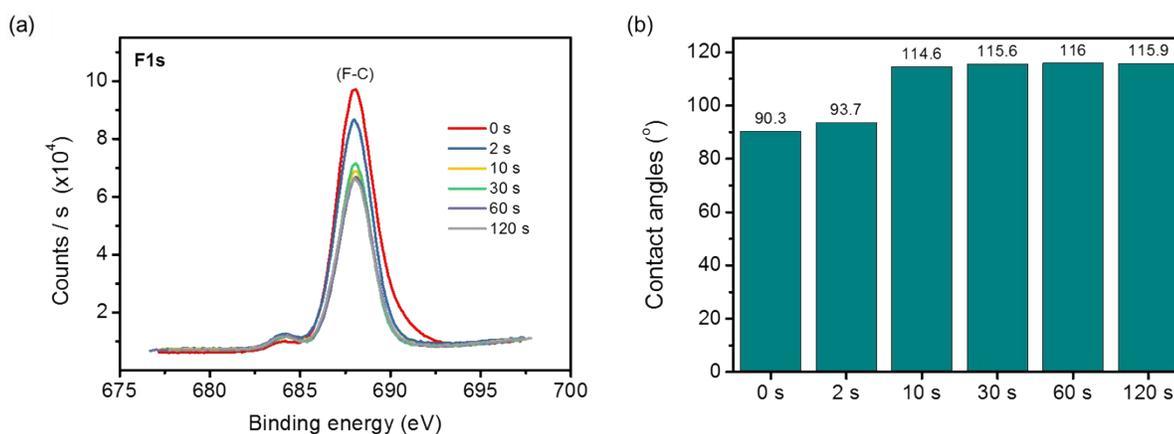
**Figure S4.** (a) HR-XPS scans of F1s on the FC10PA-treated Co substrate by the rinse time of 0, 2, 10, 30, 60, and 120 s. (b) The plot of water contact angles on the FC10PA-treated Co substrate by the rinse time of 0, 2, 10, 30, 60, and 120 s.
