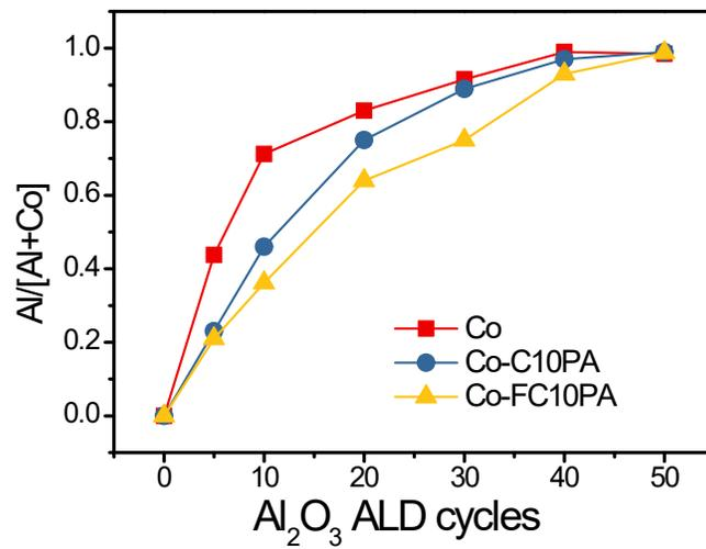
**Figure S5.** XPS composition analysis on the surfaces of Co, Co-C10PA, and Co-FC10PA after different cycles of Al<sub>2</sub>O<sub>3</sub> ALD using O<sub>3</sub> as co-reactant.
