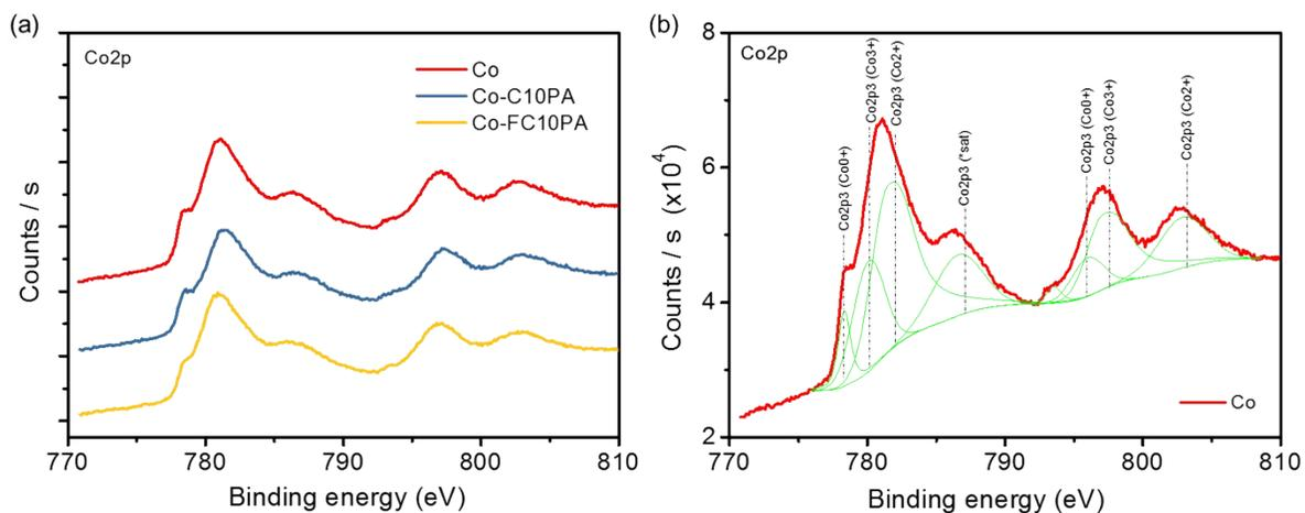
**Figure S2.** (a) HR-XPS scans of Co<sub>2</sub>p on a pristine Co wafer and Co wafers treated by C10PA and FC10PA. (b) HR-XPS scans of Co<sub>2</sub>p on a pristine Co wafer with best fitting and component peaks.
