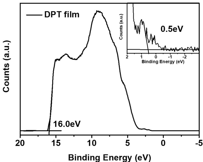
**Fig S3** UPS spectrum of DPT film. HOMO energy level is calculated according to the following equation: HOMO (vs. vacuum conditions) =  $-(E_{\text{photon}} - \text{width of UPS spectra})$ , where  $E_{\text{photon}}$  denotes the excitation energy of He I (21.22 eV)
