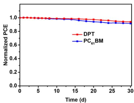
**Fig S6** Storage stability of devices under an atmosphere of nitrogen with DPT or PC<sub>61</sub>BM as the electron transporting material
