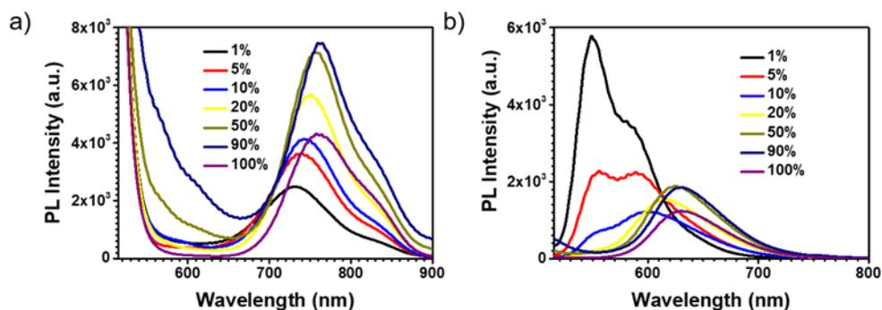
**Fig S8** Photoluminescence of PMMA film doped with a) DPT or b) PDI with different mass fraction.
