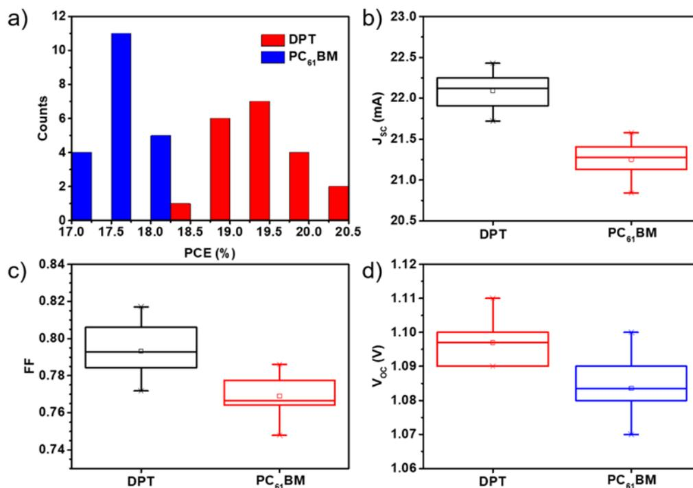
**Fig. S4** a) The PCE distributions of perovskite solar cells with PC<sub>61</sub>BM and DPT as ETMs. b-d) The corresponding photovoltaic parameters statistic
