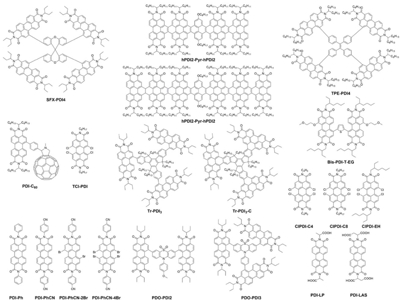
**Fig S5** Molecular structures of PDI derivatives as ETMs in PSCs
