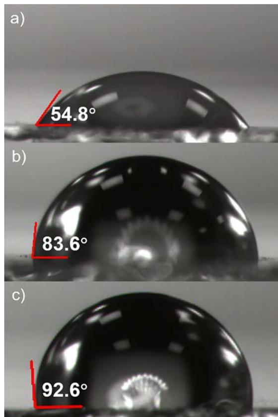
**Fig S7** Water contact angles of (a) perovskite film, (b) PC<sub>61</sub>BM covered perovskite film, and (c) DPT covered perovskite film, respectively
