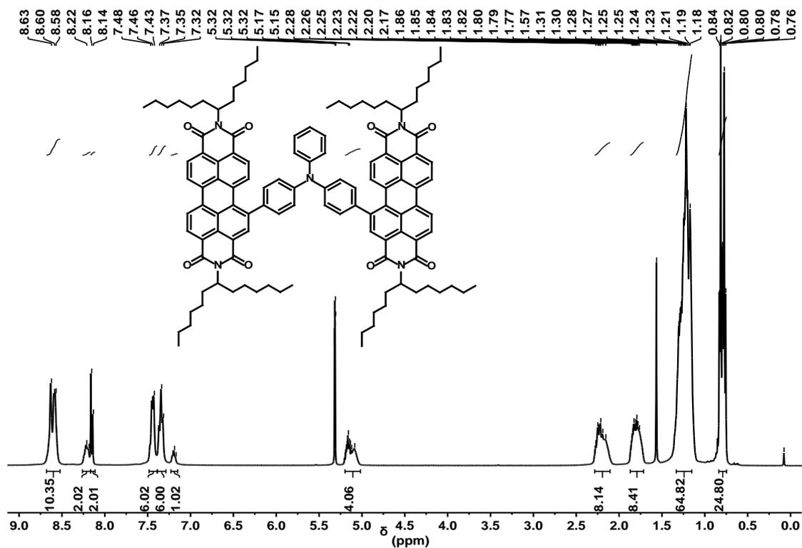
Figure S1  $^1\text{H}$  NMR spectrum of DPT with dichloromethane- $d_2$  as solvent
