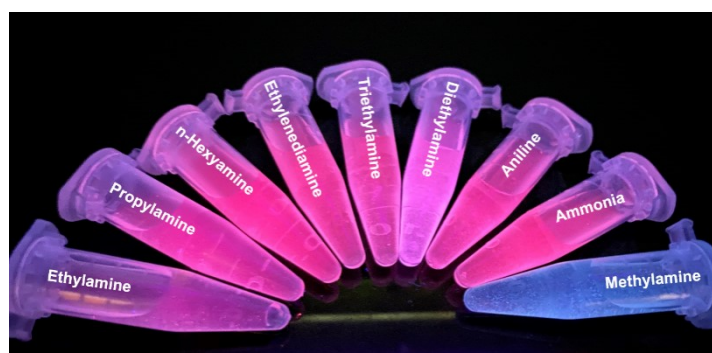
Figure S9. Photos of Eu@Tt-TPA with MA or a series of aliphatic amines, aniline and ammonia under 310 nm UV-light irradiation. The concentrations of MA and a series of aliphatic amines, aniline and ammonia were 10^{-2} M.
