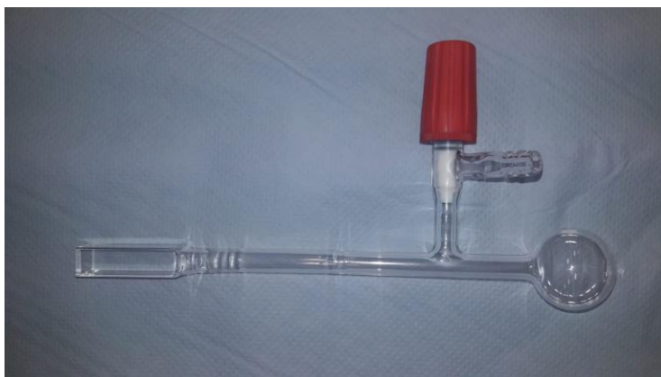
Figure S3: Photograph of a Schlenk-cuvette used for the preparation of deoxygenated solutions for photon upconversion studies.
