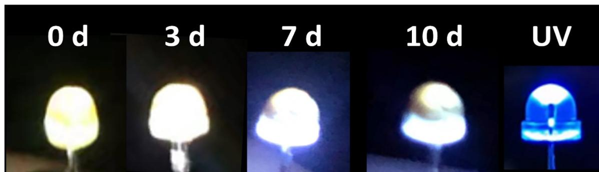
**Figure S14.** The change of WLED working continuously for 10 days
